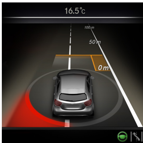
Figure 53 Breakup of the execution phase due to a fast approaching vehicle from behind
