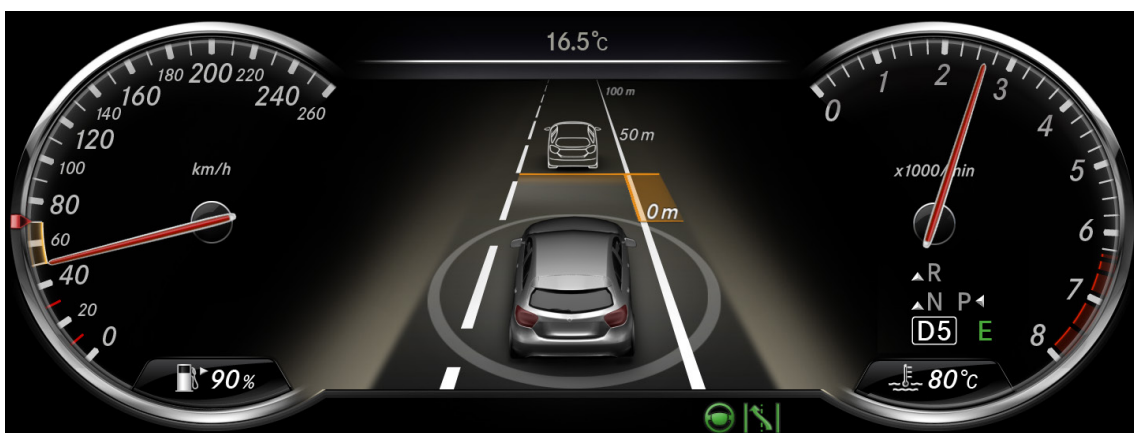
Figure 49 Lane markings and ring around ego-vehicle serve as feedback for the availability of the semi-automated lane change assistant
