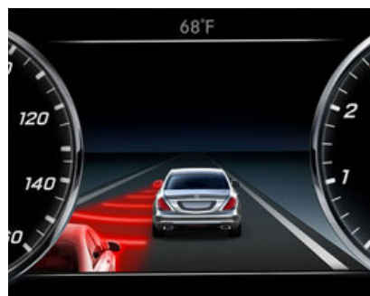
Figure 12 Mercedes-Benz active blind spot assistant
