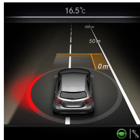
Figure 54 Breakup of the execution phase due to an approaching vehicle from the far-adjacent lane
