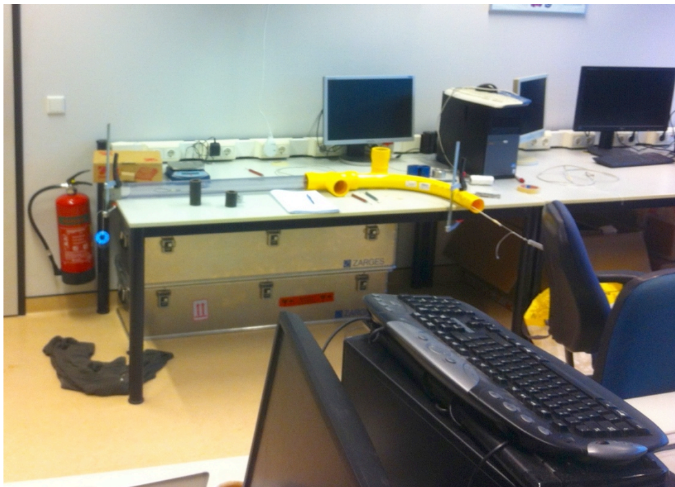
Figure 4: Test setup to determine the coefficient of friction in radius and miter bends; with on the left the weight for tension and on the right the force gauge attached to the cable.
