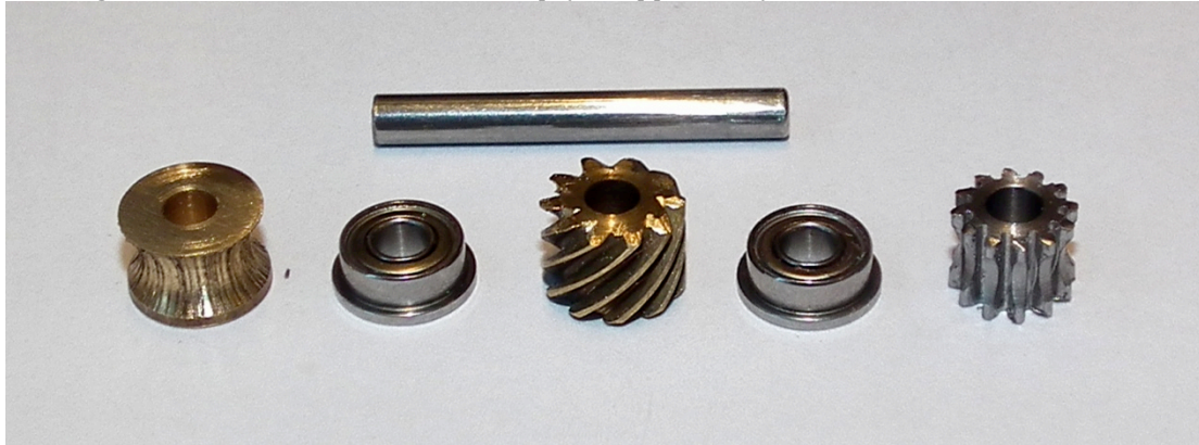
Figure 31: The shaft of the cable feeding module, on the left a pulley constructed on the lathe at TCO.
