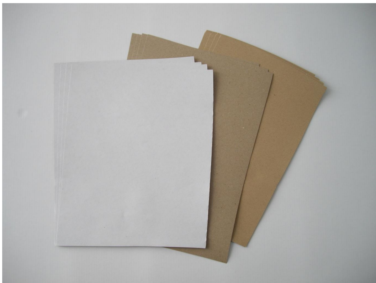
Figure F20 | VPK paper samples: 135 white testliner (left), 135 fluting (middle) and 135 testliner (right)
