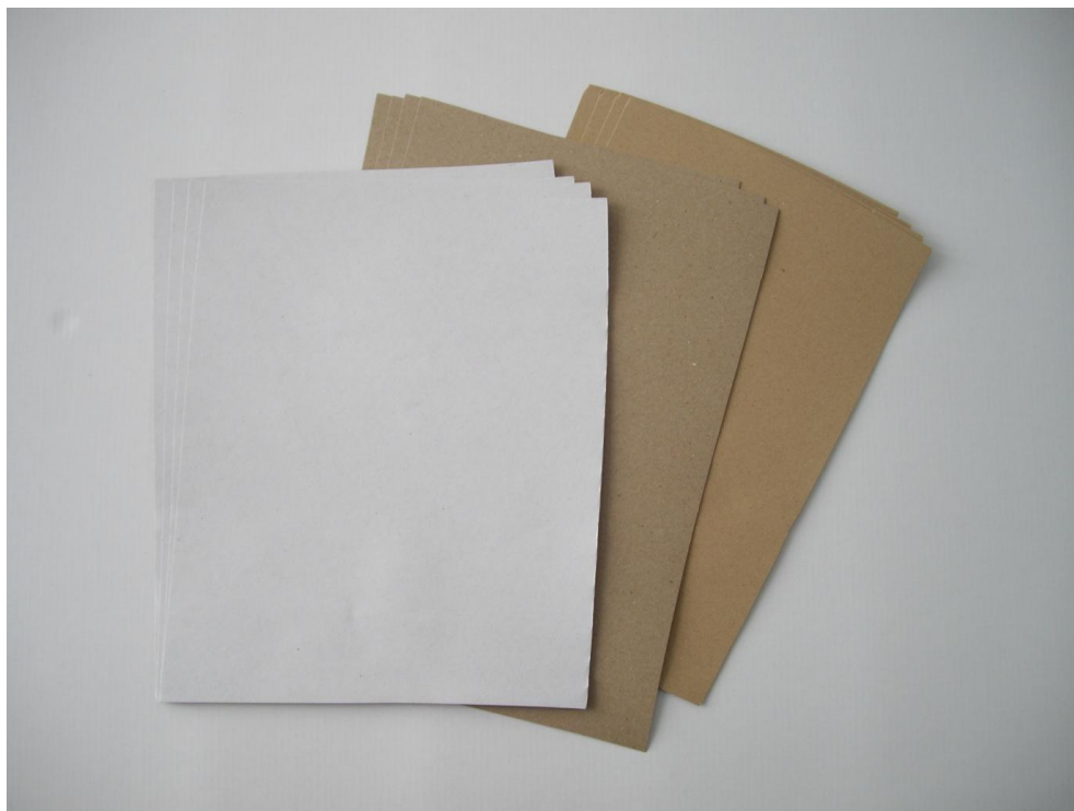
Figure 4.16 | VPK paper samples: 135 white testliner (left), 135 fluting (middle) and 135 testliner (right)
