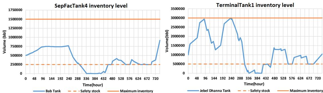
Figure 11: Inventory levels of a separation facility and a terminal storage tank for the unstable demand case
