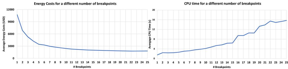
Figure 23: Energy costs and CPU time for a different number of breakpoints
