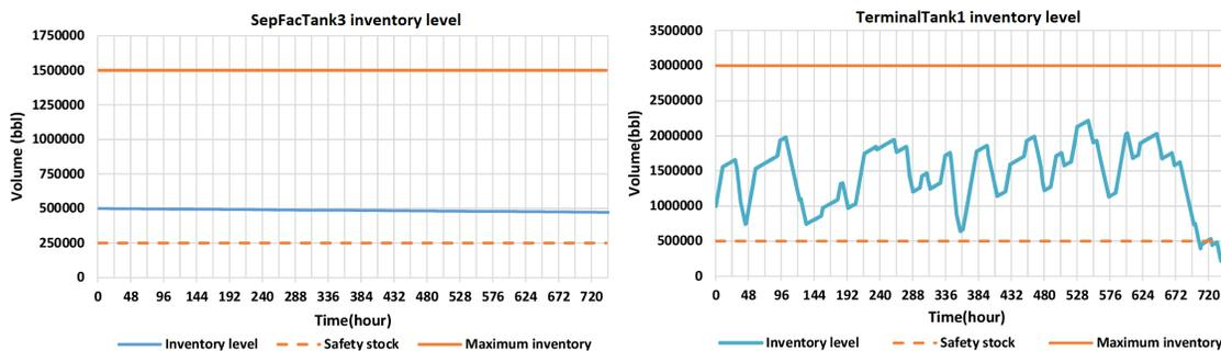
Figure 10: Inventory levels of a separation facility and a terminal storage tank for the stable demand case
