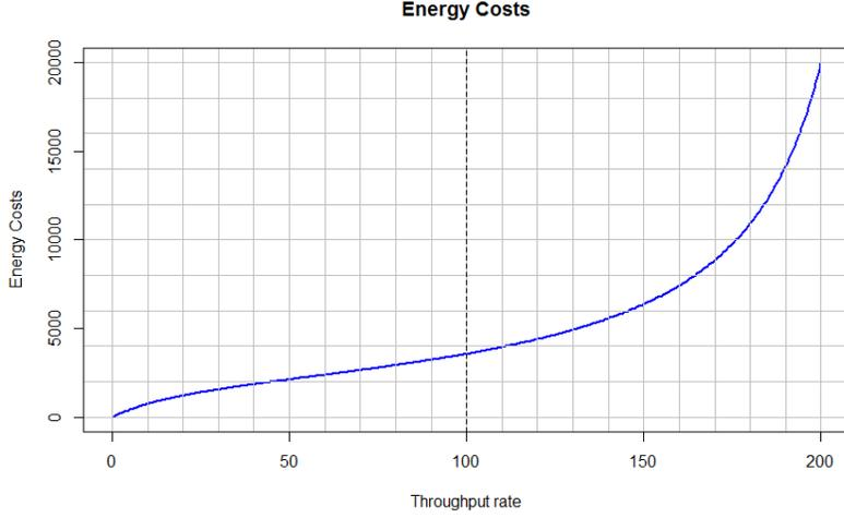
Figure 6: Energy costs of the example pump at different throughput rates
