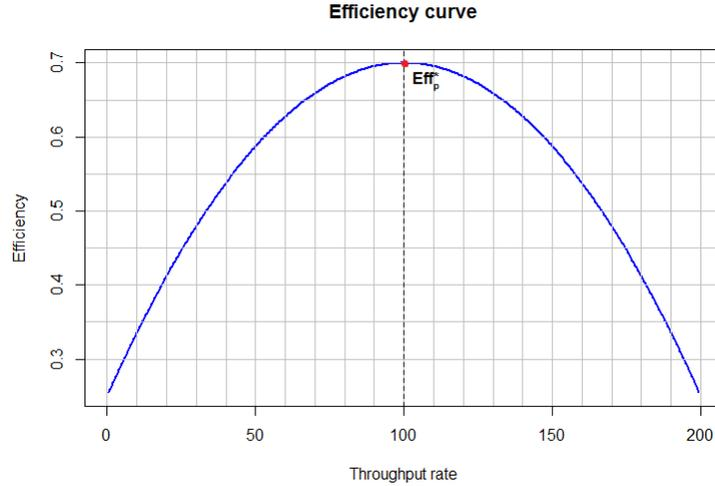
Figure 22: The efficiency curve of the example pump
