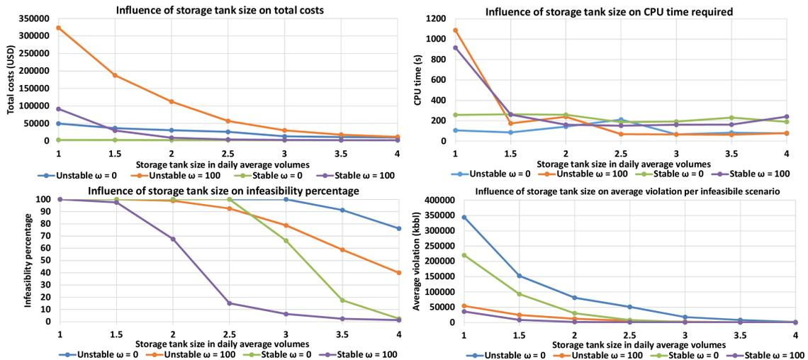
Figure 25: Storage tank volumes based on average daily volume experiment results
