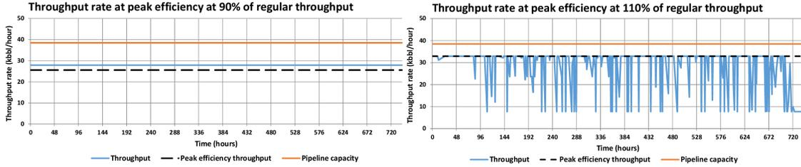
Figure 21: Difference in throughput in the optimal solution for a peak efficiency throughput below and above the regular throughput
