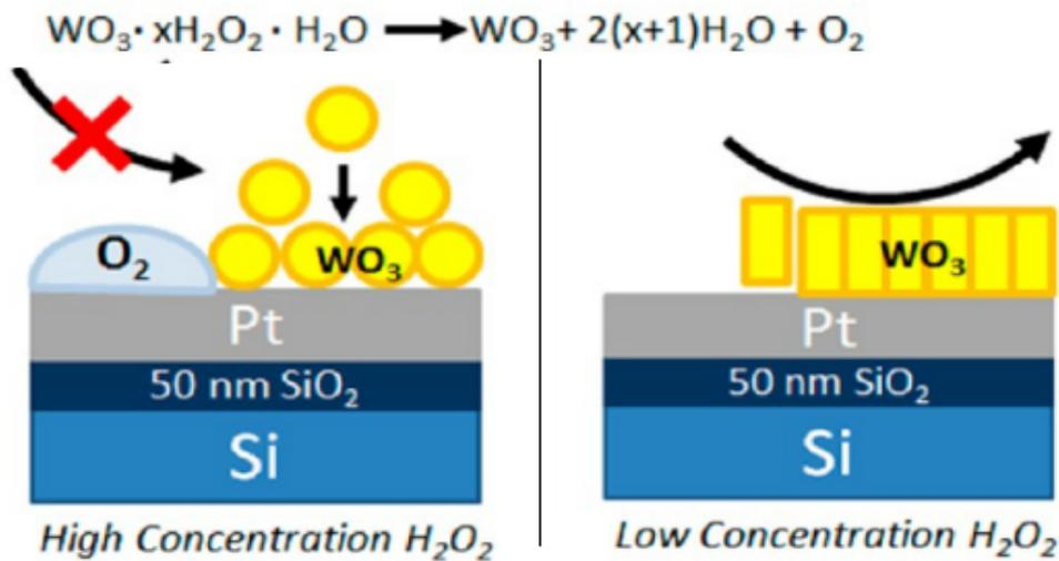
FIGURE 3.3:  $\text{WO}_3$  growth with and without excess of  $\text{H}_2\text{O}_2$ [8]
