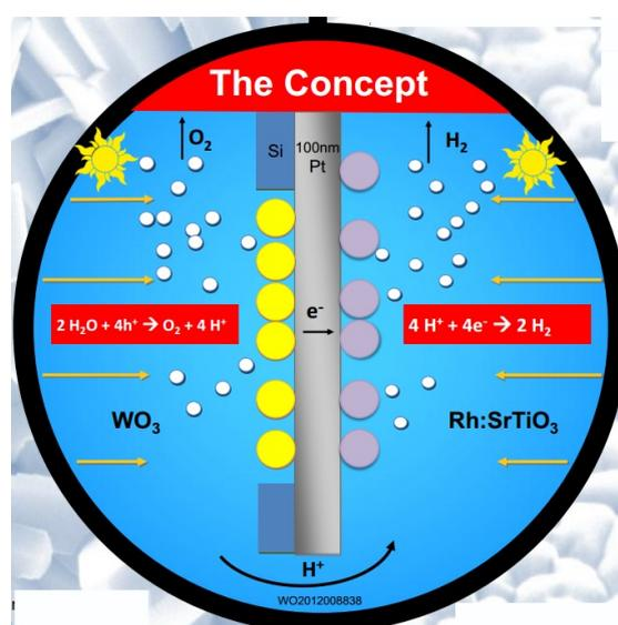
FIGURE 2.6: Water splitting cell lay-out[14]
