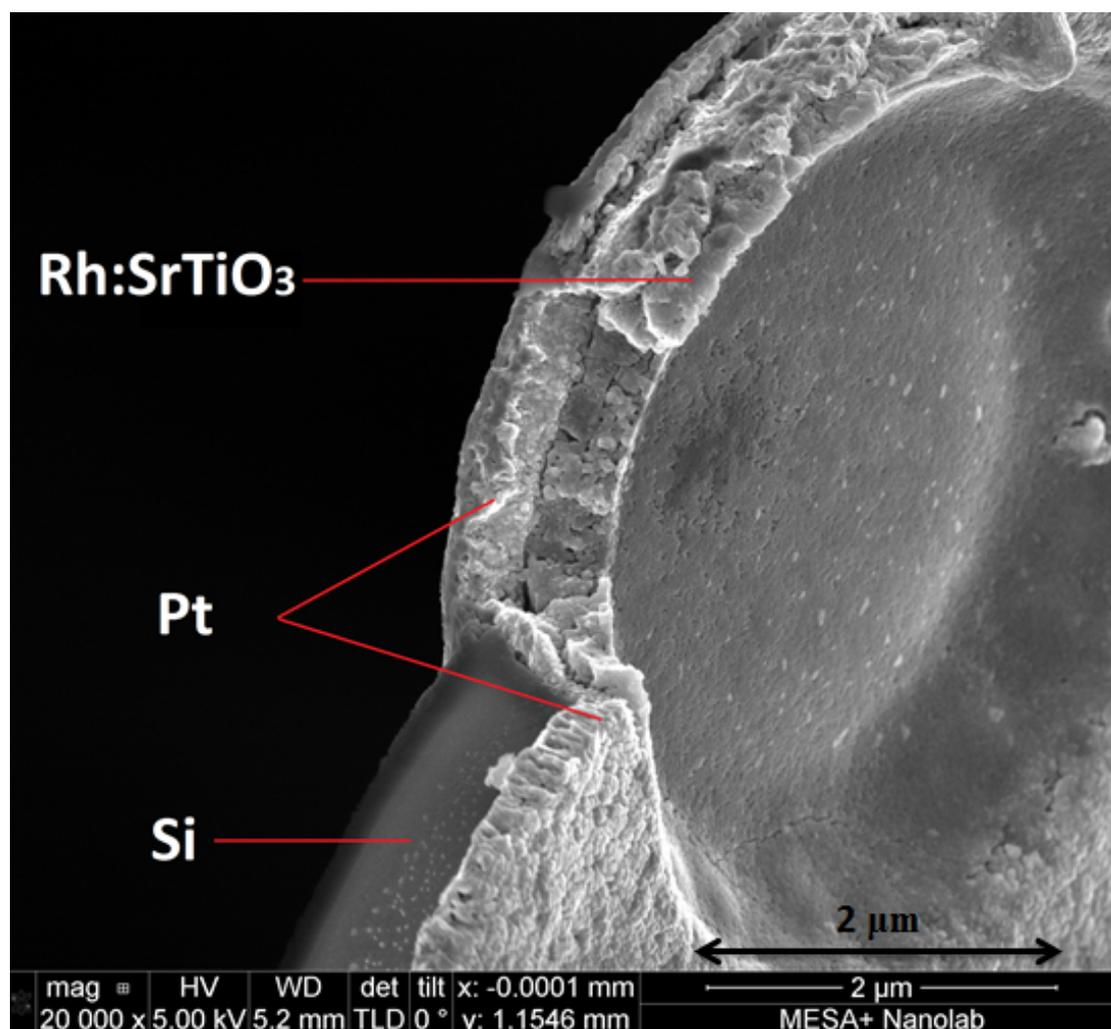
FIGURE 4.7: SEM image of peeled in membrane with SrTiO<sub>3</sub>:Rh layer on it.
