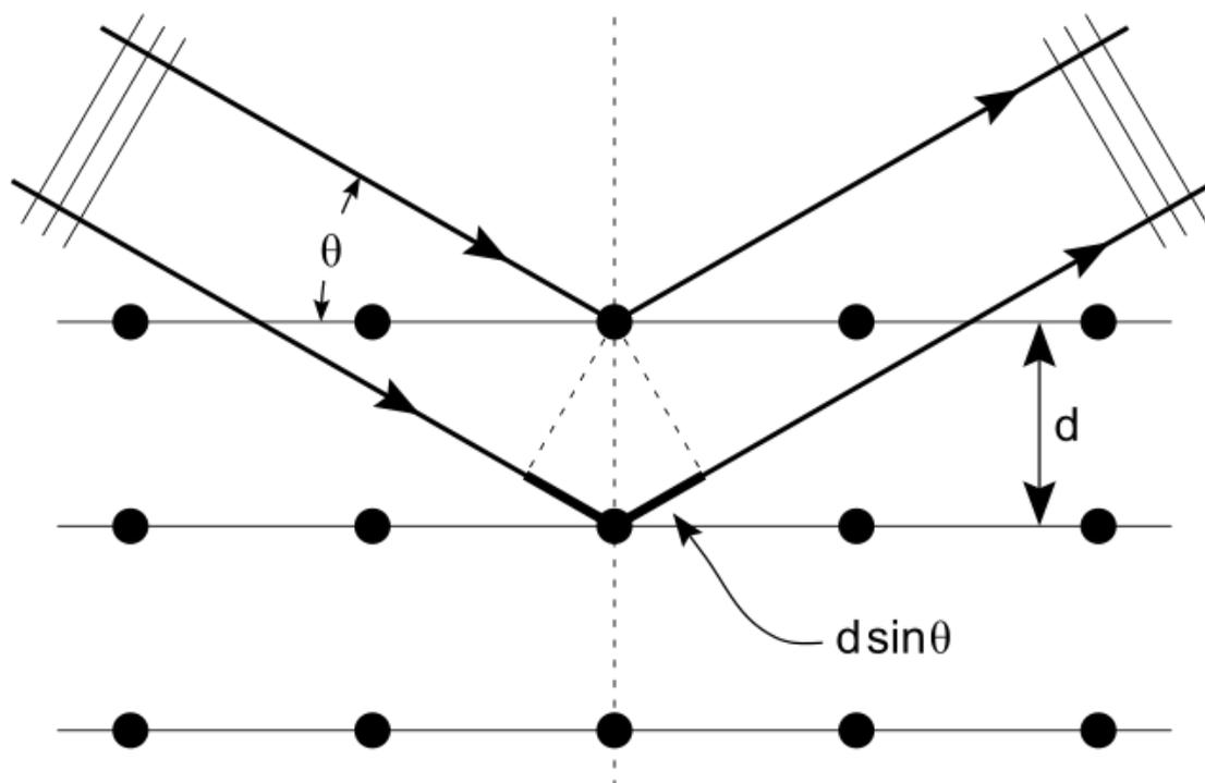
FIGURE 3.7: Bragg's diffraction
