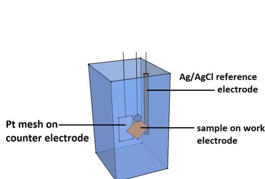
FIGURE 3.4: Set up for a cyclic voltammetry measurement
