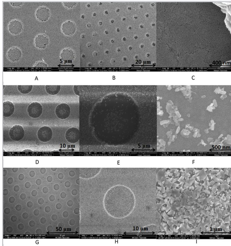
FIGURE 4.8: A, B: SEM images of the top of two different membranes with 5 layers  $\text{SrTiO}_3\text{:Rh}$  grown on top of it and with  $\text{WO}_3$  grown on it. C: zoomed in SEM image of the same membrane B. D, E, F: SEM images of a membrane with 3 layers of  $\text{SrTiO}_3\text{:Rh}$  and covered while  $\text{WO}_3$  grown on it. G, H, I: SEM images of a membrane with 5 layers of  $\text{SrTiO}_3\text{:Rh}$  and covered while  $\text{WO}_3$  grown on it.
