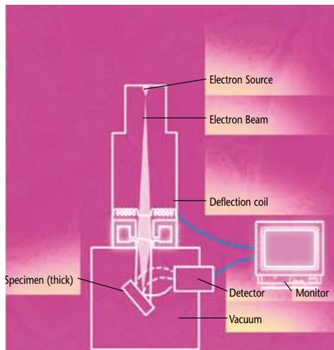
FIGURE 3.8: Schematic diagram of a SEM[11]
