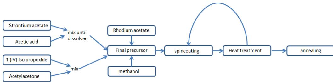
FIGURE 3.2: Diagram of SrTiO<sub>3</sub>:Rh synthesis
