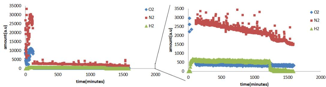
FIGURE 4.12: GC measurement of a membrane with WO<sub>3</sub> and SrTiO<sub>3</sub>:Rh integrated on it.
