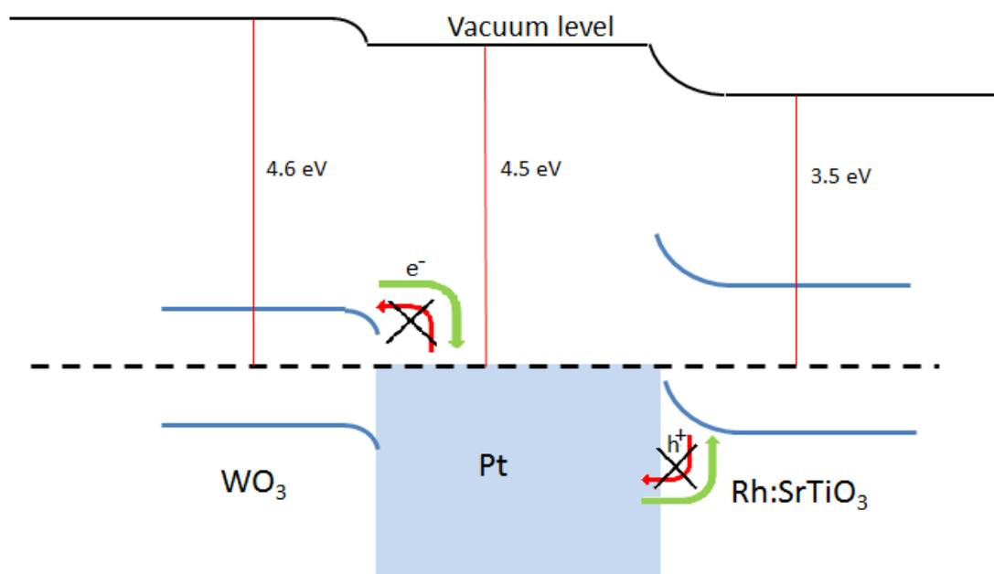
FIGURE 4.11: Band diagram of WO<sub>3</sub>, Pt and SrTiO<sub>3</sub>:Rh and there interfaces
