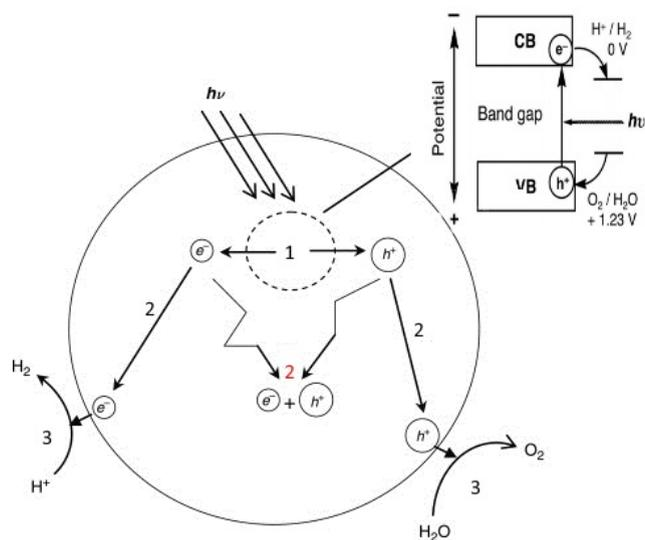
FIGURE 2.1: Three steps of water splitting. 1: photon absorption and creation of an electron-hole pair. 2: separation of the electron-hole pair and migration to the surface. 3: half reaction with water.[1], [2]
