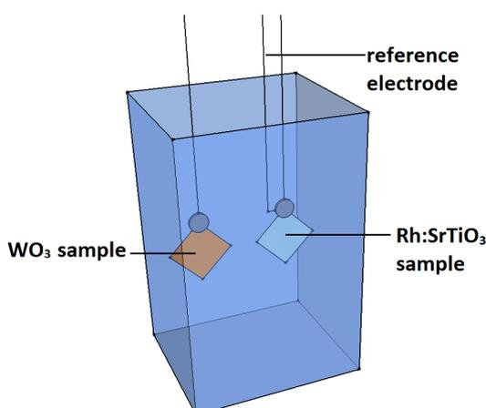
FIGURE 3.5: Set up for a chronoamperometry cell
