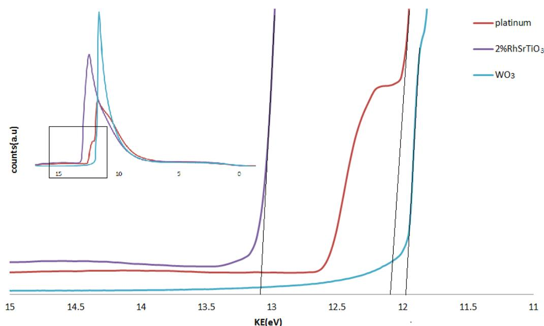
FIGURE 4.10: UPS measurement, amount of electrons counted Vs the kinetic energy of these electrons
