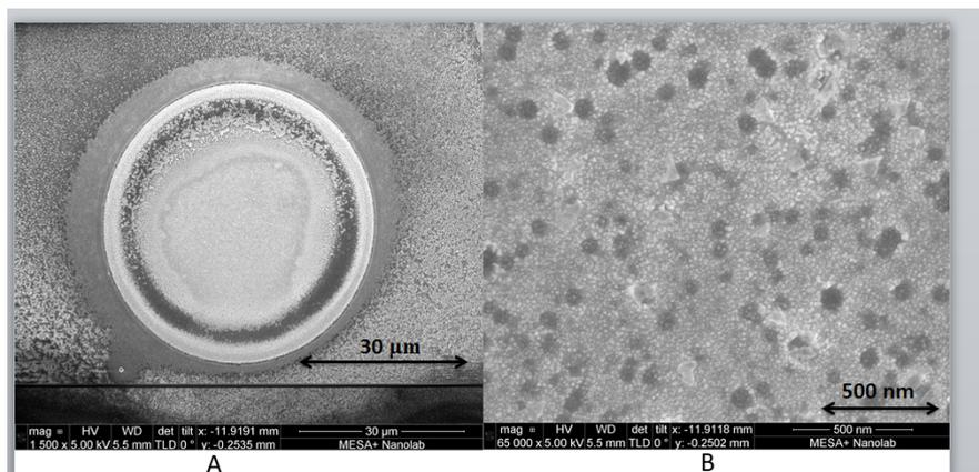
FIGURE 4.9: Back side of the membrane with  $\text{WO}_3$  growth.
