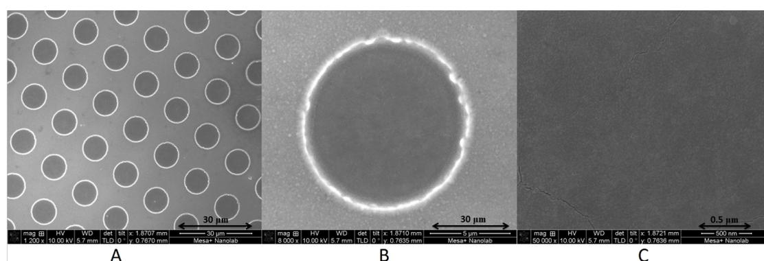
FIGURE 4.6: SEM images of the top of a membrane with three layers of SrTiO<sub>3</sub>:Rh layer on it.
