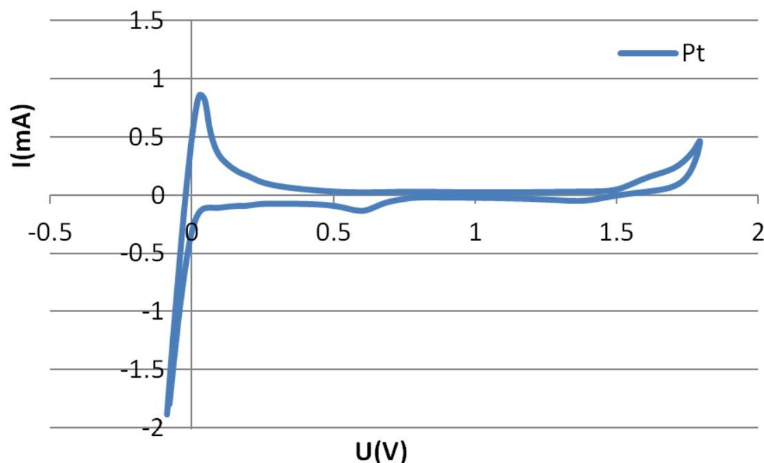
FIGURE 3.6: Cyclic voltammetry measurement of a Pt sample
