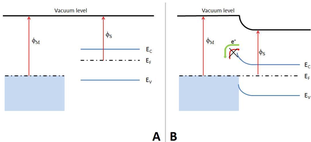
FIGURE 2.5: Band diagram of a metal-semiconductor interface. A: Metal and semiconductor are not touching so the bands don't bend. B: Metal and semiconductor touch and the bands of the semiconductor bend.
