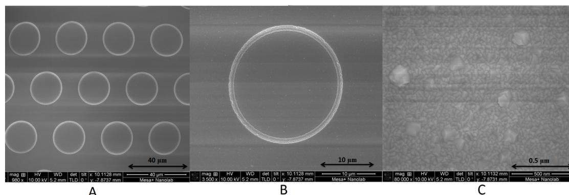
FIGURE 4.5: SEM images of the top of a clean membrane.
