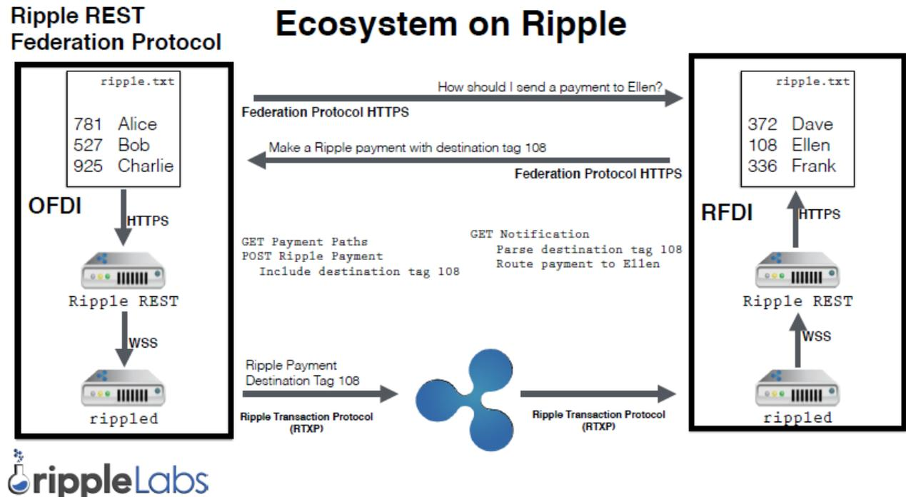
Figure 6.6 Federation protocol facilitating the use of destination tags. Source: Ripple Labs
