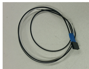
(f) Connector for four of the six pwm pins.
