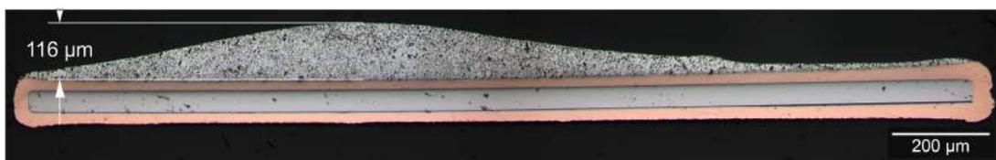
**Figure 2.11:** Crosssection of the 2-mm wide tape with solder of a voltage tap.
