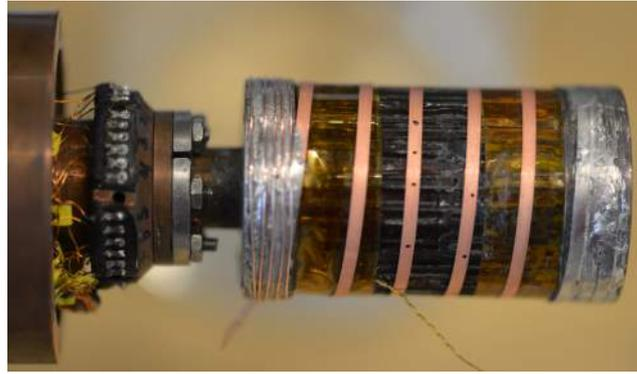
**Figure 2.5:** The sample holder, with a 2 mm tape soldered to copper terminals. On the left terminal a bare NbTi wire can be seen, used for reinforcement. Visible next to the left terminal, near the flange, are the contact pads for the electrical connections. The black underneath the tape is the embedded heater with its ribbed support structure.
