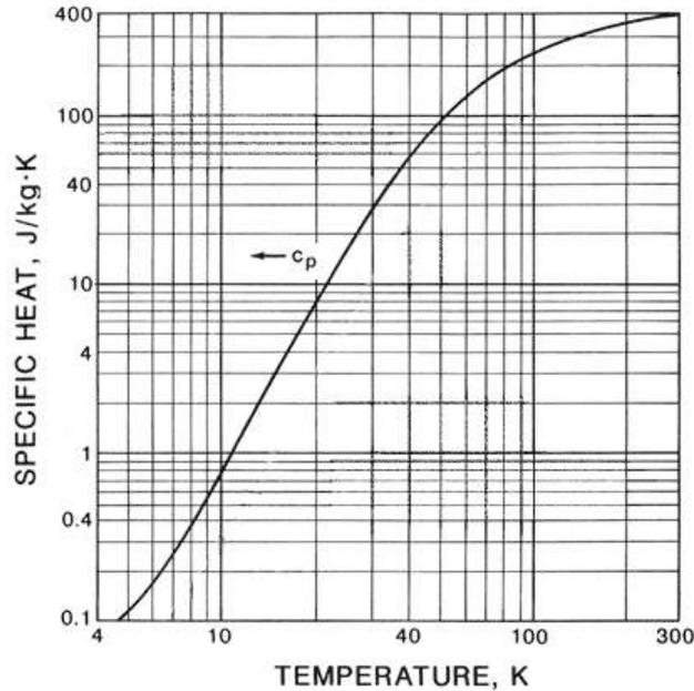
**Figure 1.3:** Specific heat of copper. Below the 100 K, the specific heat drops rapidly.
