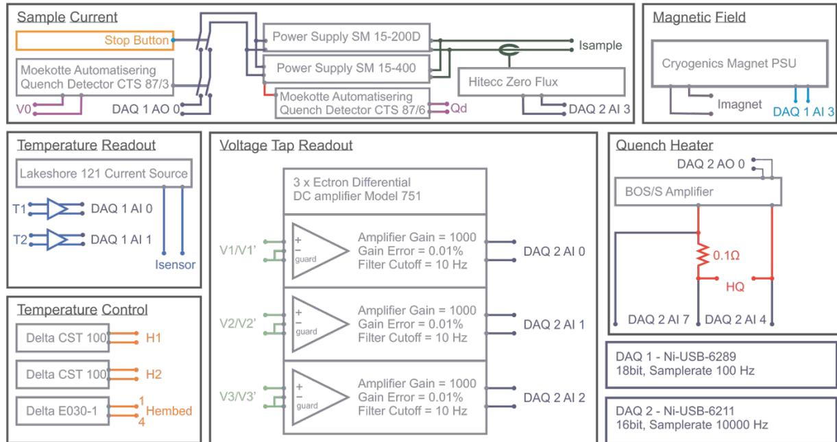
Figure 4: Schematic overview of the instrumentation and its connections.
