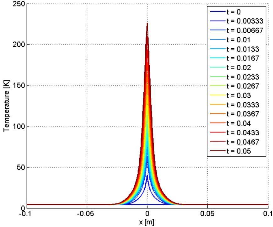
**Figure 4.4:** Temperature development of a simulated quench, with  $B = 14\text{T}$  at  $T = 4.2\text{ K}$  and  $I = 170\text{ A}$ .
