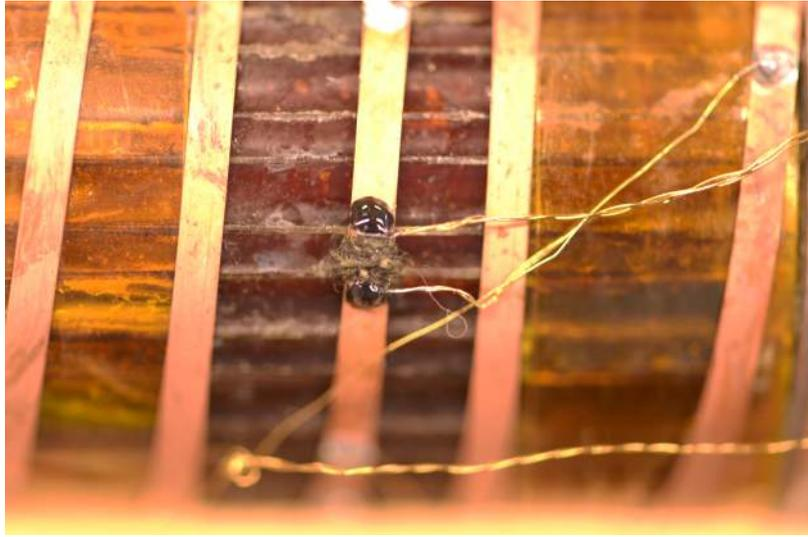
**Figure 2.3:** The quench heater, fixed to the tape with nylon wire. Thermal grease was applied between the tape and the heater. Epoxy secures it lateral position.
