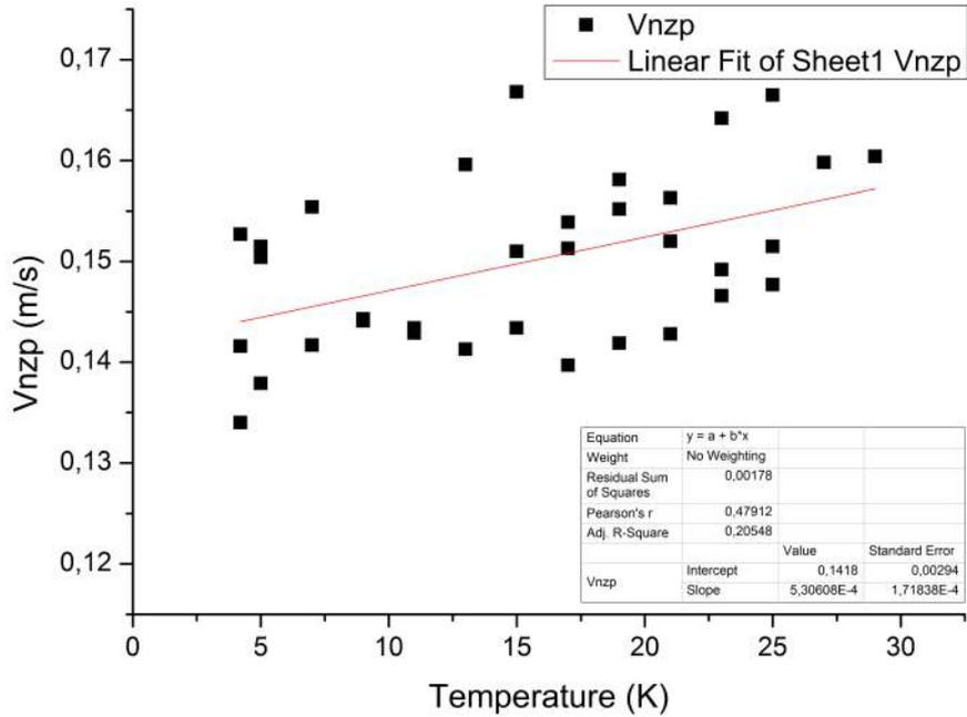
**Figure 3.5:** The temperature dependence of  $V_{nzp}$  at a constant current of 170 A. A fitted linear trend line is added, with a slope of  $(5.3 \pm 1.7) \times 10^{-4}$  m/s per Kelvin. Four points fell out of the error margin and were excluded.
