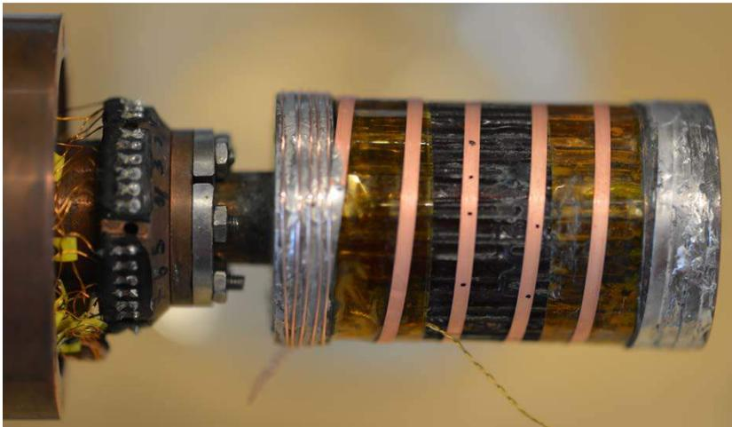
Figure 11: 2 mm tape with element position markings, soldered to the current leads and on the left, reinforced with niobium titanium wire.
