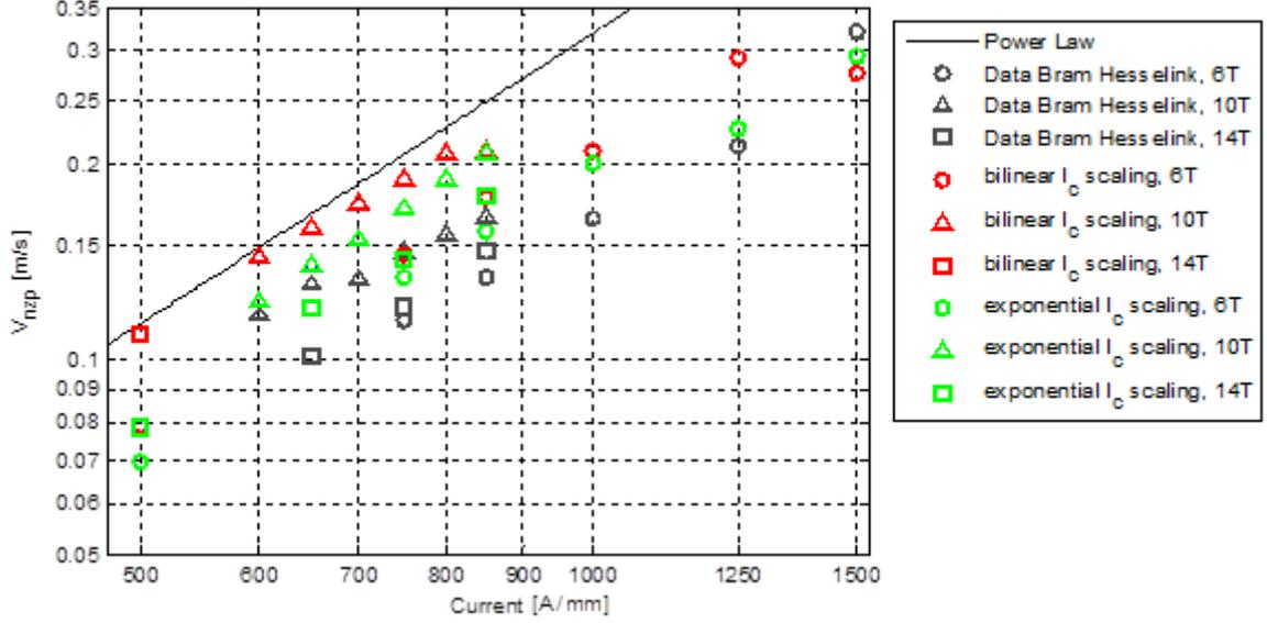
**Figure 4.7:** Results from the simulation of current dependent  $V_{nzp}$ . For  $T = 4.2$  K at  $B = 6$  T;  $T = 25$  K at  $B = 10$  T and  $T = 23$  K at  $B = 14$  T.
