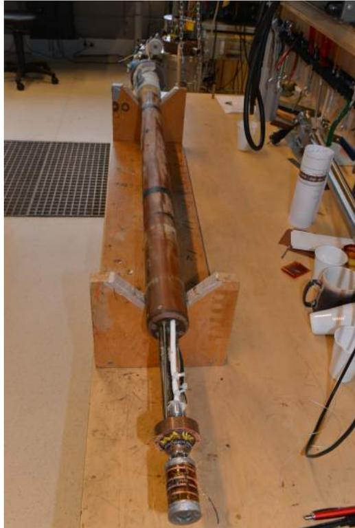
**Figure 2.4:** The low temperature insert
