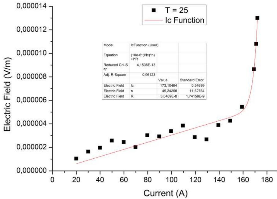
**Figure B.1:** Critical current measurement of the 2-mm tape at  $B = 14$  T and  $T = 25$  K. Found  $I_c = 173$  A with  $N = 45$ .
