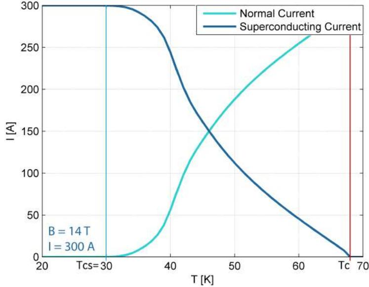
**Figure 4.3:** Example of current sharing in the 4-mm tape.  $T_{cs}$  is at  $T = 30$  K.  $T_c$  is at  $T = 68$  K.
