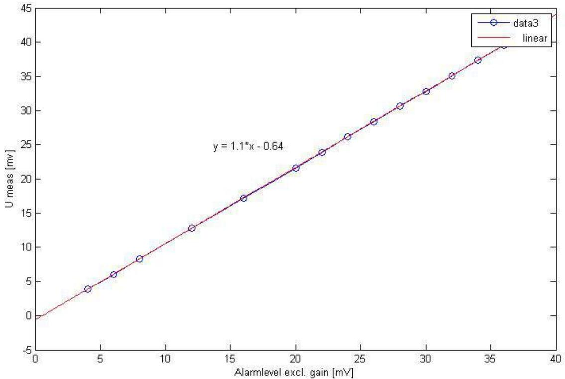
Figure 8: For CTS 87/3. The input voltage versus the trigger voltage set by the alarm level. The line should be  $x = y$ .
