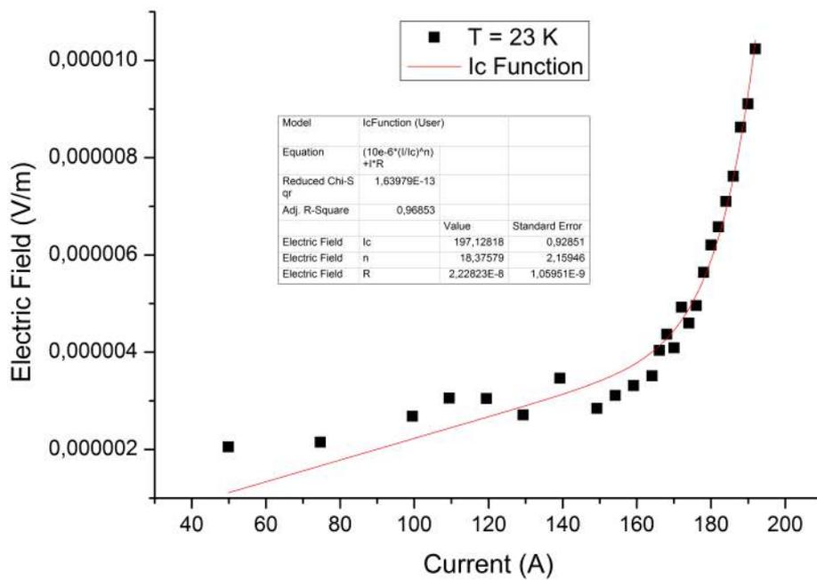
**Figure B.2:** Critical current measurement of the 2-mm tape at  $B = 14$  T and  $T = 23$  K. Found  $I_c = 197$  A with  $N = 18$ .
