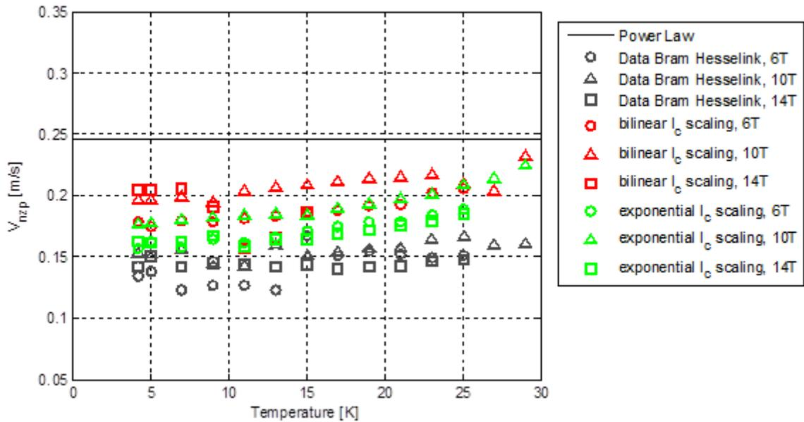
**Figure 4.6:** Results from the simulation of temperature dependence of  $V_{nzp}$ , at a constant current of  $I = 85$  A/mm width.
