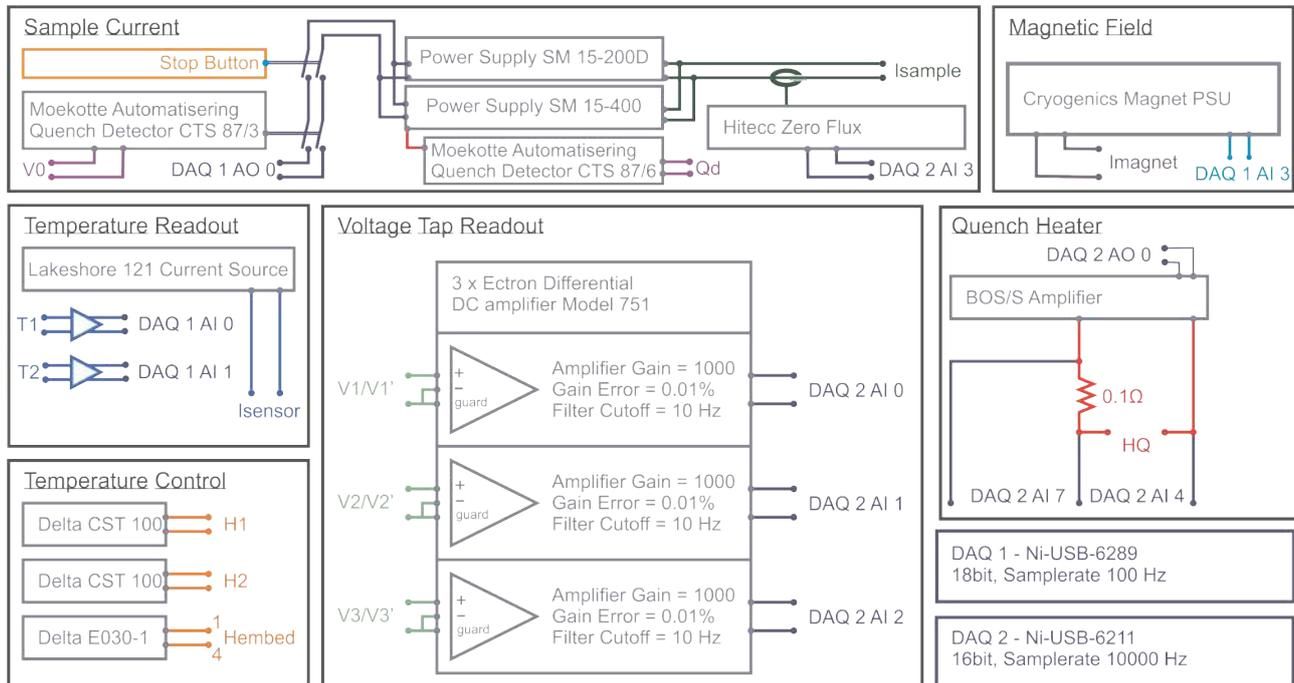
**Figure 2.6:** Scheme of the setup configuration and connections
