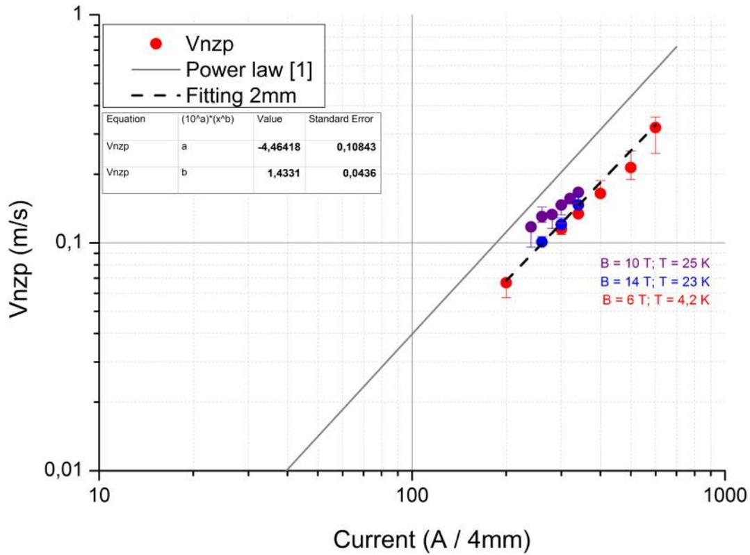
**Figure 4.8:** Measured  $V_{nzp}$  compared with the earlier found current dependence
