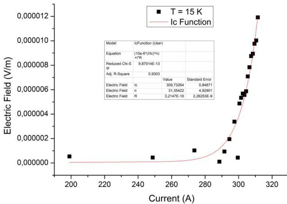
**Figure B.6:** Critical current measurement of the 2-mm tape at  $B = 14$  T and  $T = 25$  K. Found  $I_c = 310$  A with  $N = 31$ .
