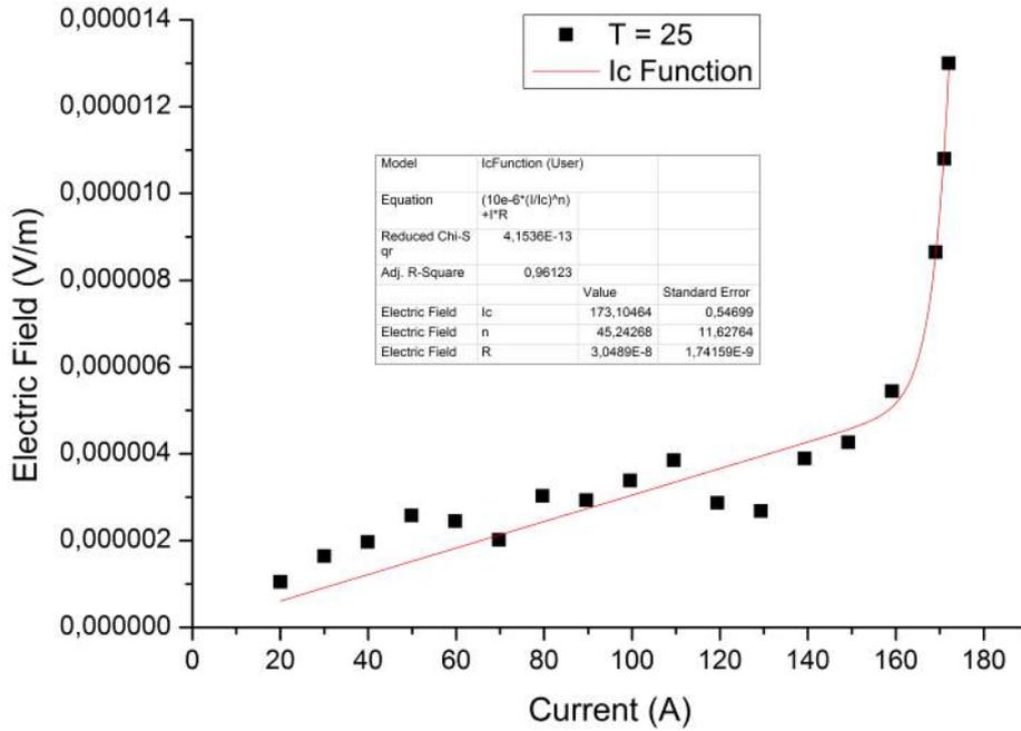
**Figure 2.8:** Graph of a critical current measurement at  $T = 25$  K and  $B = 14$  T.
