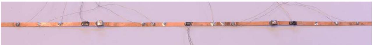
**Figure 2.2:** A tape sample with the voltage taps, heaters and temperature sensor housings.
