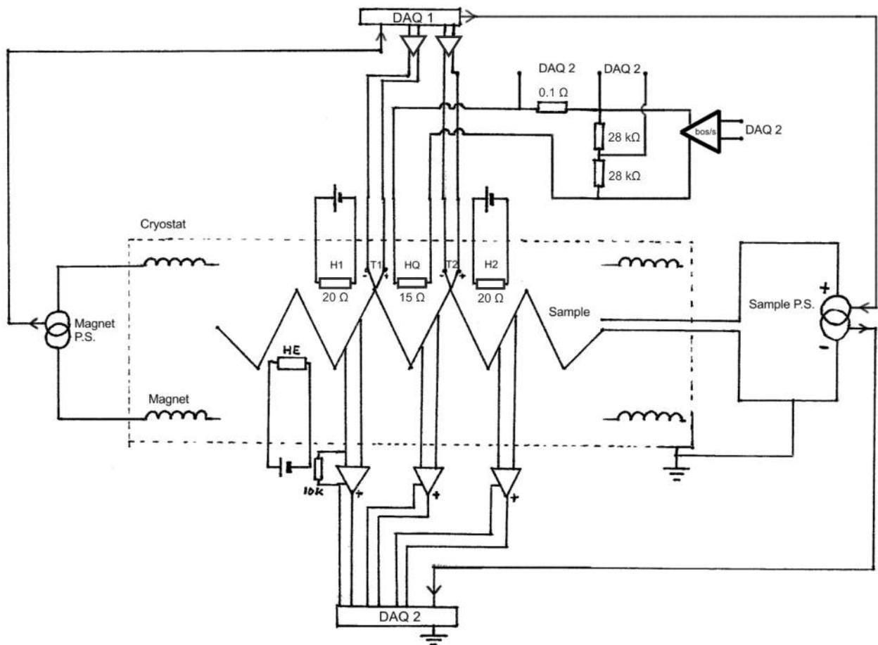
**Figure 2.7:** The electrical schematic of the NZP-experiment. A connection between the amplifier input and output is established to prevent a voltage buildup with the ground. The grounding of DAQ 2 was disconnected.
