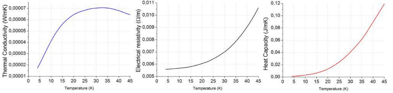
**Figure 4.1:** Calculated average material properties for the 2-mm wide REBCO tape [9]. Plotted against temperature are the electrical resistivity ' $\rho$ ', the thermal conductivity ' $k$ ' and the heat capacity ' $C$ '.
