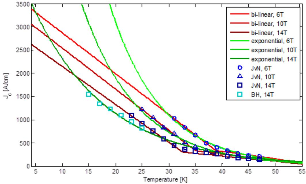
**Figure 4.5:** Critical current density values at different magnetic field strengths, used for the simulations. The points represent the measured values, the lines show the values using the fitted scaling relations. JvN stands for the measurements of the 4-mm wide tape, BH for the 2-mm wide tape data collected in this work. Behind the name in the legend the value of the magnetic background field is indicated.
