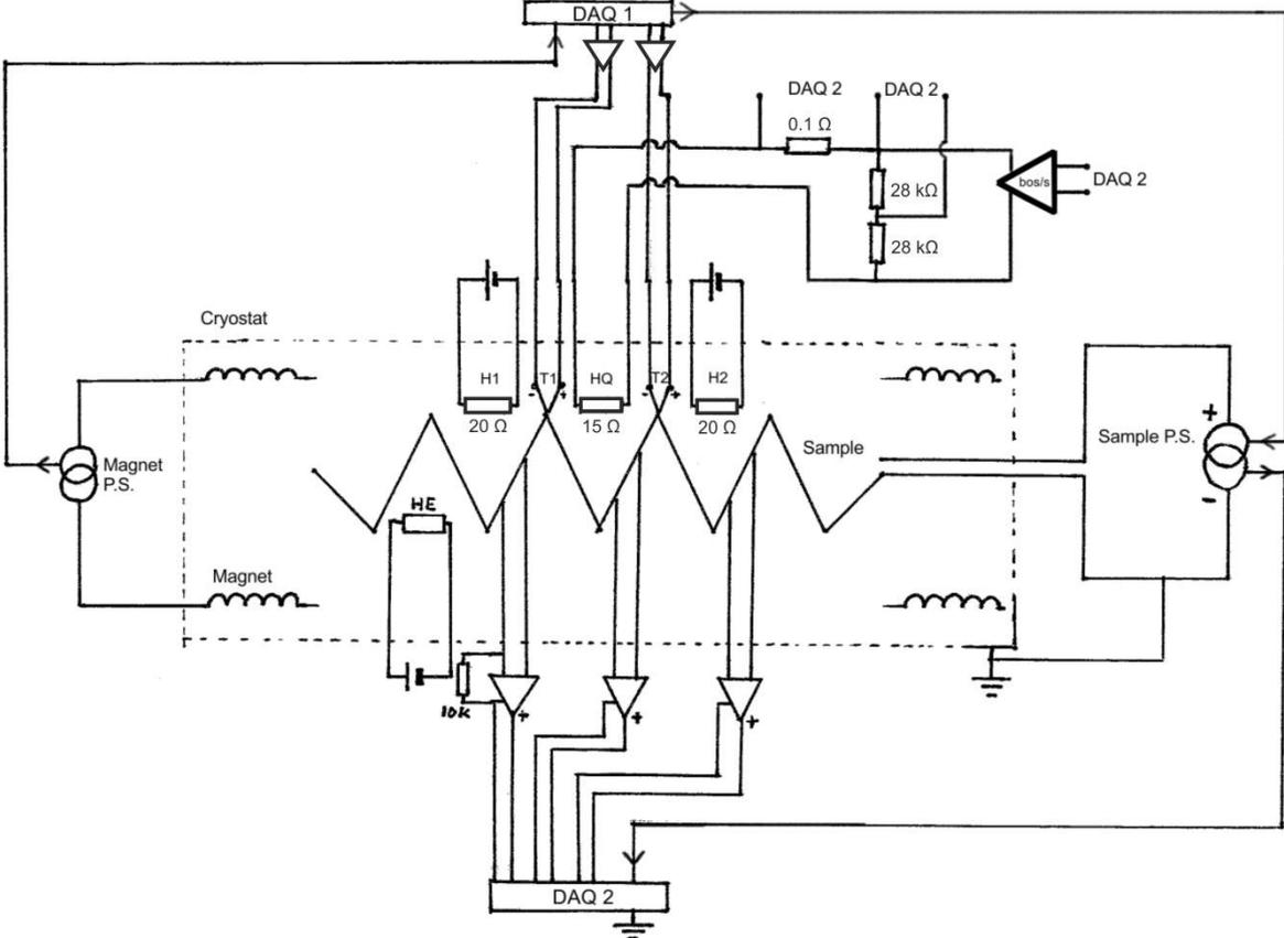
Figure 5: Electrical scheme of the setup. To overcome grounding problems, the DAQ 2 was disconnected from ground.
