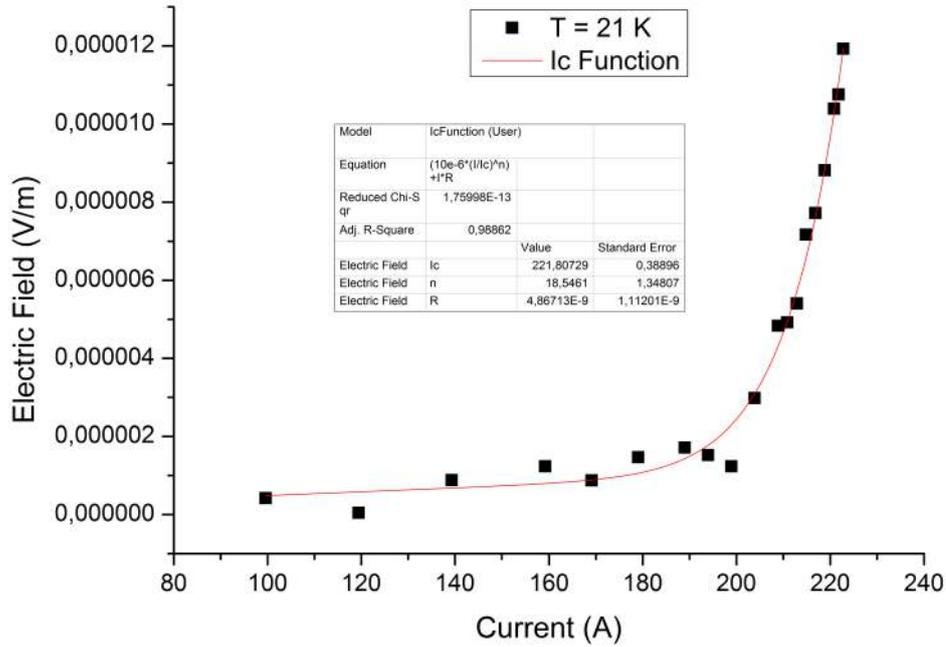
**Figure B.3:** Critical current measurement of the 2-mm tape at  $B = 14$  T and  $T = 21$  K. Found  $I_c = 222$  A with  $N = 19$ .
