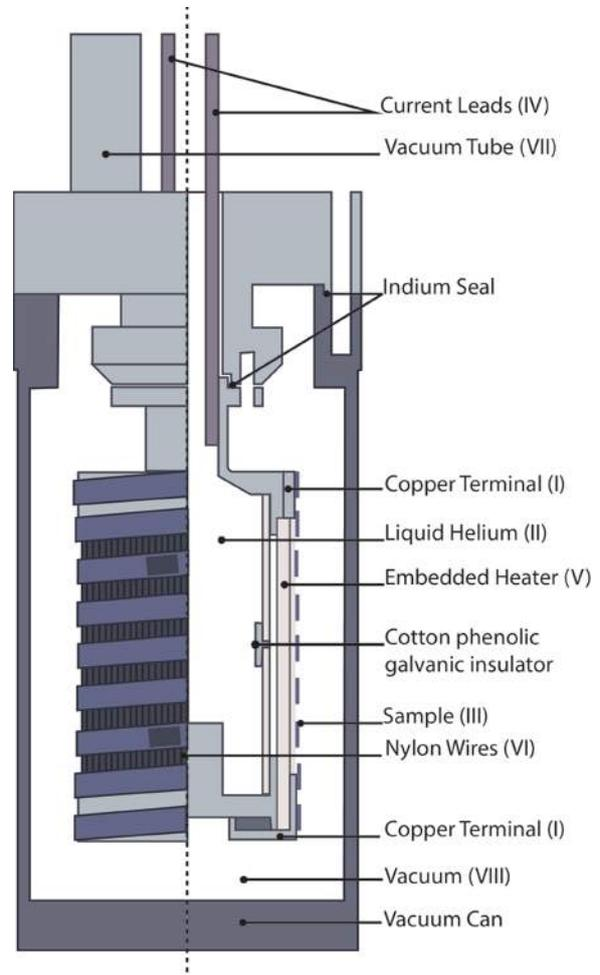
Figure 3: Schematic of the sample holder.
