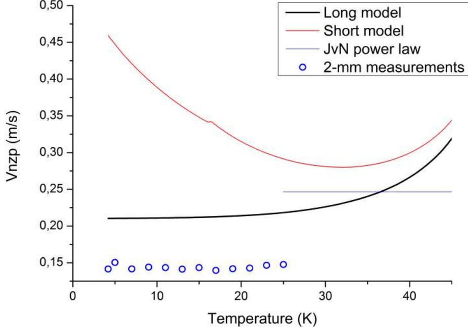
**Figure 4.2:** Comparison of the 'short model' prediction Eqn. 4.2, the 'long model' prediction Eqn. 4.3, the 'power law' behavior observed in the 4 mm tapes [JvN] and the present data on the 2-mm tape. The models are considered at an operating current of 173 A and a magnetic field of 14 T.
