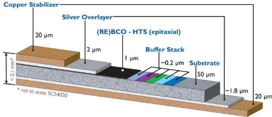
**Figure 2.1:** The buildup of the used REBCO tape manufactured by Superpower inc.
