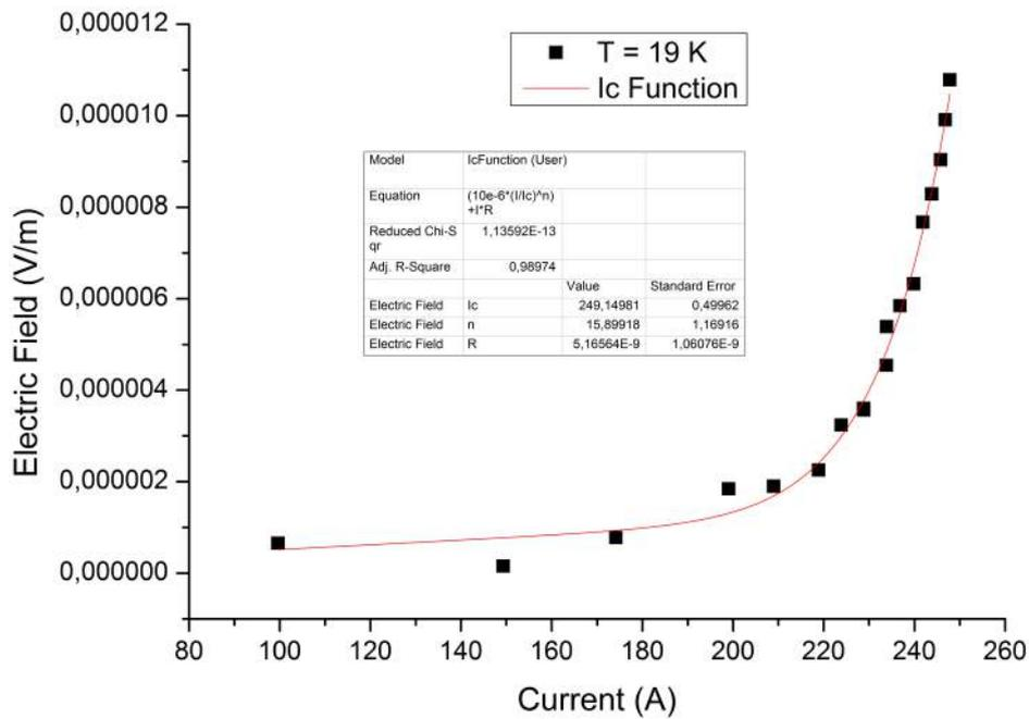
**Figure B.4:** Critical current measurement of the 2-mm tape at  $B = 14$  T and  $T = 19$  K. Found  $I_c = 249$  A with  $N = 16$ .
