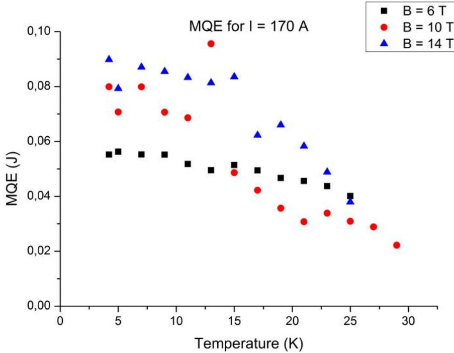
**Figure 3.2:** The dependence of the MQE on temperature and magnetic field, measured at a constant current of 170 A. The numbers are not adjusted for heater inefficiency.
