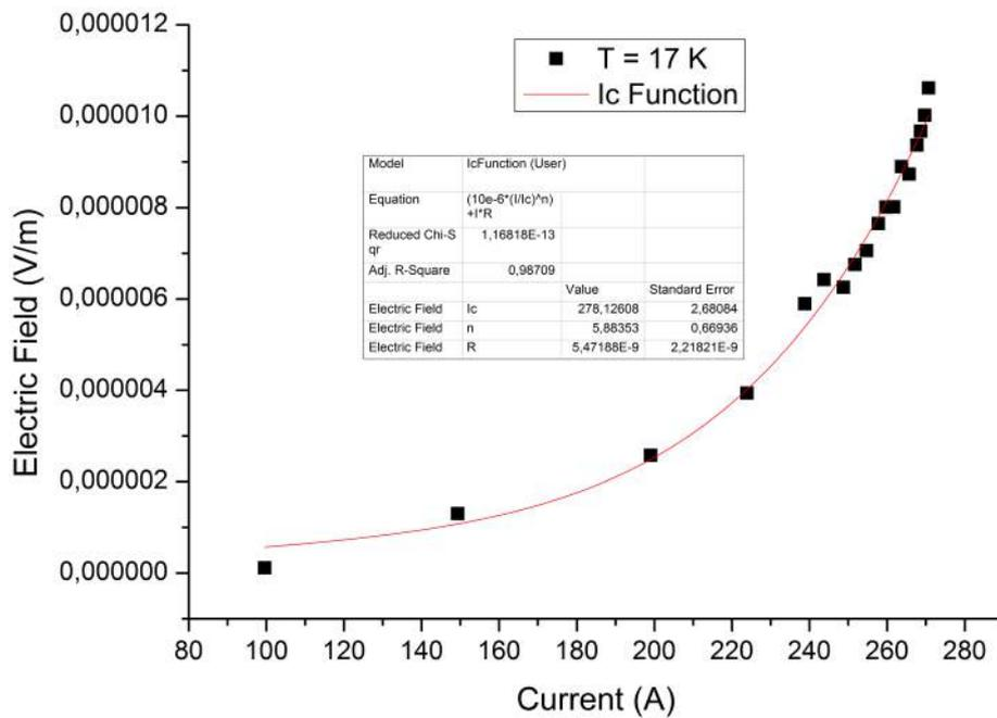
**Figure B.5:** Critical current measurement of the 2-mm tape at  $B = 14$  T and  $T = 17$  K. Found  $I_c = 278$  A with  $N = 6$ .
