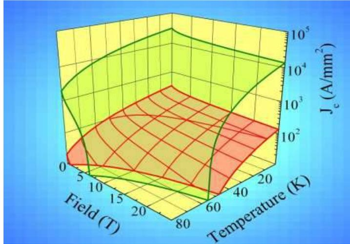
**Figure 1.2:** The critical surface of YBCO. The green top surface is for a perfect sample. The red surface is the practical engineering current density.
