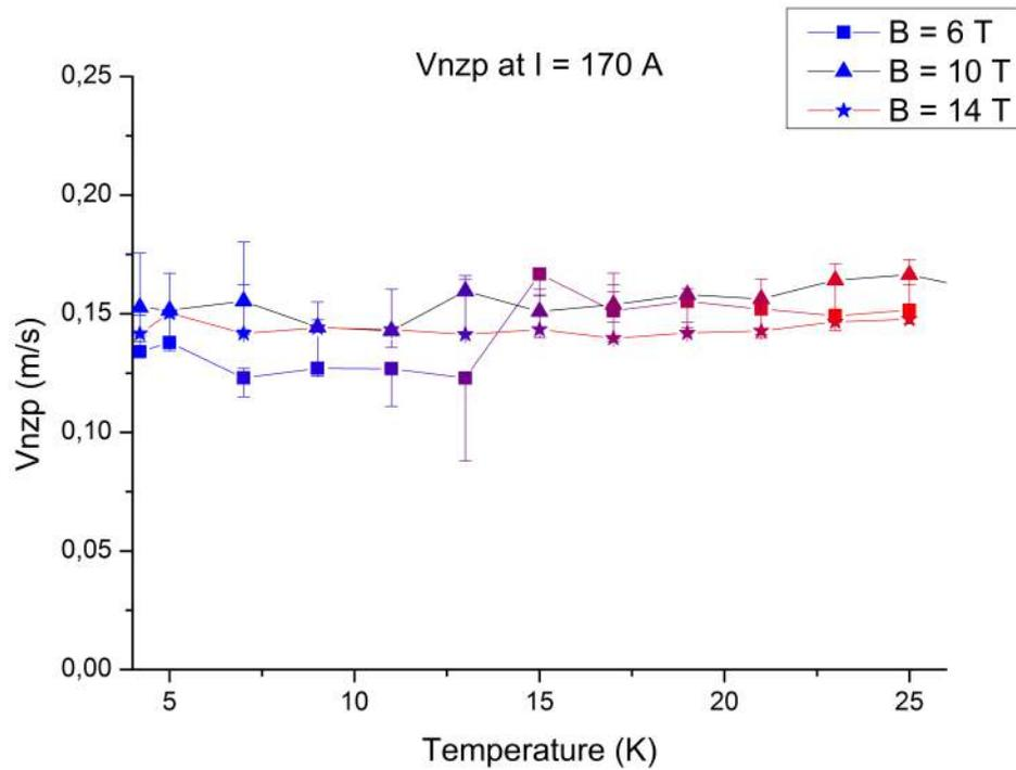
**Figure 3.4:** Vnzp versus temperature. The velocity changes with 9 percent between 4.2 and 29 K. At several temperatures, the velocity at different magnetic field strengths show an overlap. The error was determined by analysing the threshold voltage (section 2.5)
