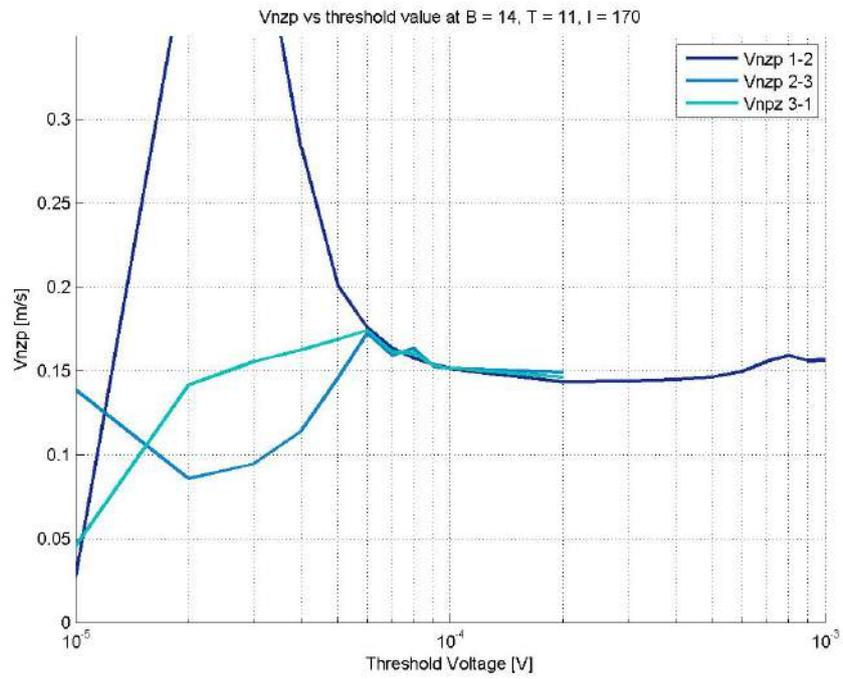
**Figure 2.10:** A profile of figure 2.9 with  $V_{nzp}$  versus threshold voltage. At a threshold voltage of  $200 \mu V$ , the signals are stable and the velocities of all taps are comparable.
