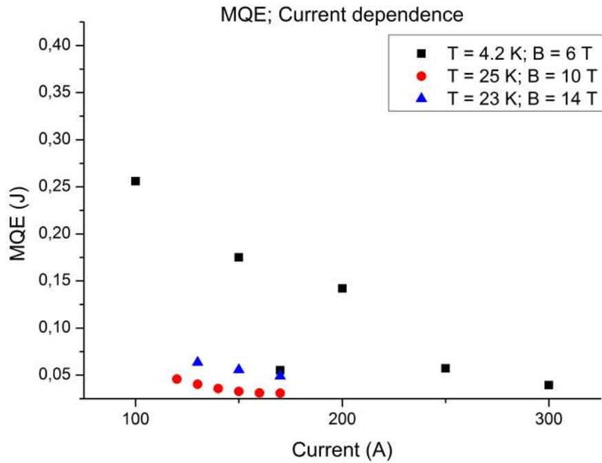
**Figure 3.3:** MQE versus sample current. The values of MQE are not compensated for any heater inefficiencies.
