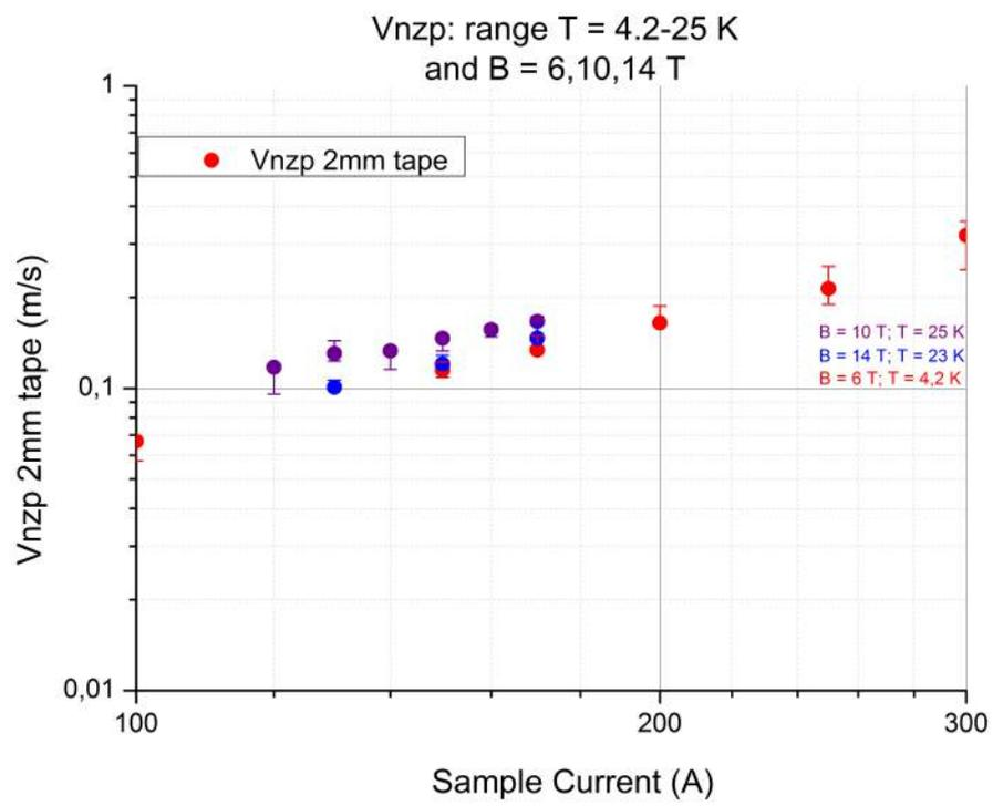
**Figure 3.6:**  $V_{nzp}$  measured versus sample current at three different combinations of magnetic field and temperature.
