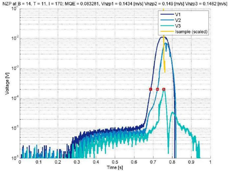
**Figure 2.9:** A clear voltage signal from a quench event.
