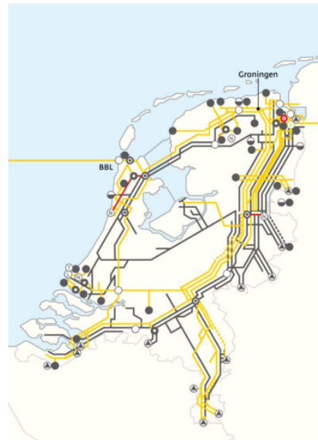
Figure 3.1: The gas transmission network in the Netherlands. In yellow the H-gas network, in black the G-gas.
