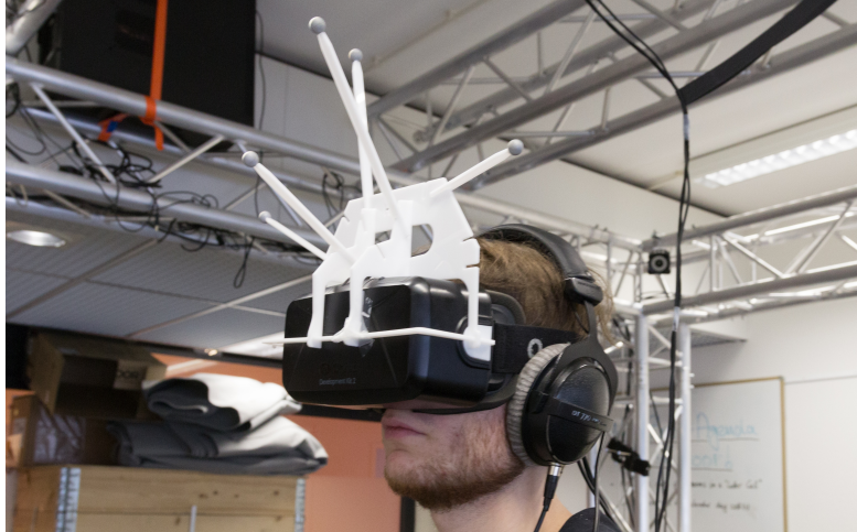
Figure 5.5.: The Head Mounted Display with retroreflective IR-markers on a plastic adapter, Headphones as worn by participants.
