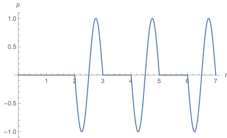
Figure 3: The return signal form a single pulse with unit frequency and unit amplitude in a single layer of unit length with unit speed of sound, full reflection at the boundaries and no attenuation.
