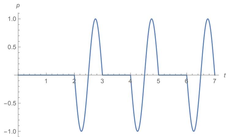
Figure 4: The return signal form a single pulse with unit frequency and unit amplitude in a two layers of half unit length with unit speed of sound, full reflection at the boundaries and no attenuation.
