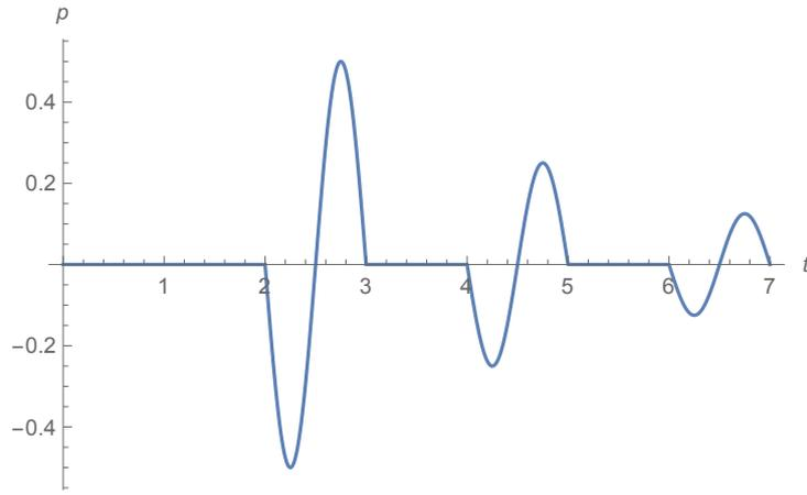
Figure 6: The return signal form a single pulse with unit frequency and unit amplitude in a single layer of unit length with unit speed of sound, full reflection at the boundaries and an attenuation factor of  $\frac{1}{2} \ln(2)$ .
