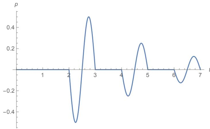
Figure 7: The return signal form a single pulse with unit frequency and unit amplitude in a single layer of unit length with unit speed of sound, full reflection at the left boundary, half reflection at the right boundary and no attenuation.
