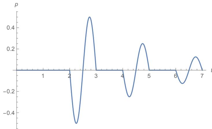
Figure 8: The return signal form a single pulse with unit frequency and unit amplitude in a single layer of unit length with unit speed of sound, full reflection at the left boundary, half reflection at the right boundary and no attenuation.
