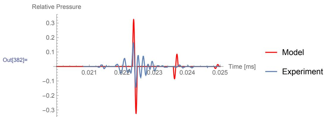
Figure 18: Comparison of result of the experiment and model of cup 3 at 6.8 MHz.
