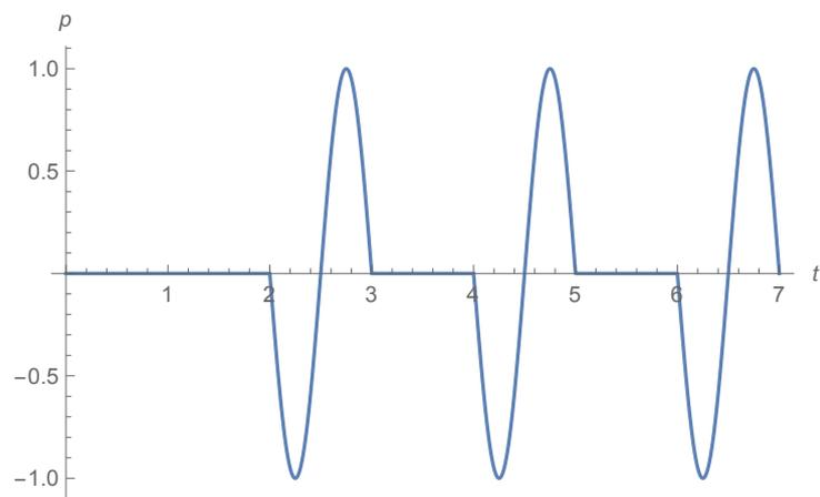
Figure 5: The return signal form a single pulse with unit frequency and unit amplitude in three layers of third unit length with unit speed of sound, full reflection at the boundaries and no attenuation.
