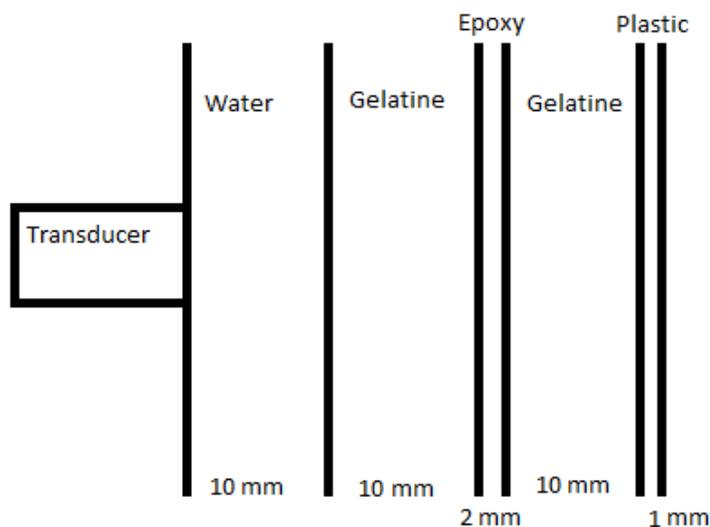
Figure 9: A schematic overview of cup 3.
