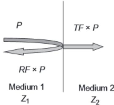
Figure 2: A schematic overview of reflection and transmission on a boundary. (Szabo 2014, p61)
