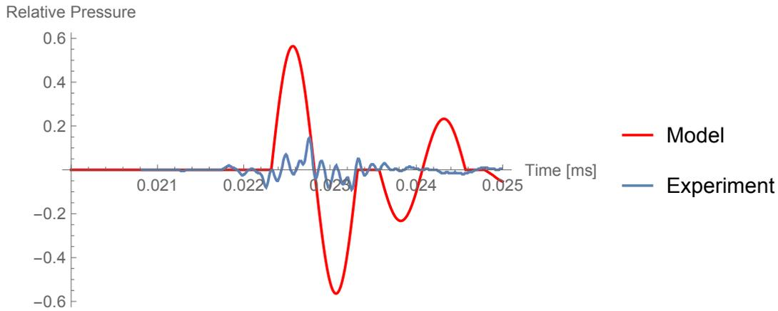
Figure 19: Comparison of result of the experiment and model of cup 3 at 1 MHz.
