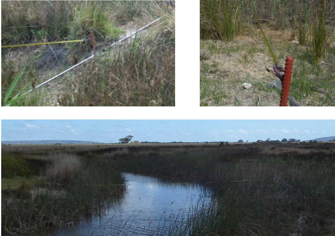
FIGURE 3.8: TAPELINE FOR MANUAL MEASUREMENTS OF CROSS SECTIONS. (ABOVE LEFT) TAPELINE AND SILVER MEASURING ROD FOR READING DEPTHS, (ABOVE RIGHT) TAPELINE WHICH HAS BEEN FIXED IN POSITION, (BELOW) OVERVIEW OF MANUAL DEPTH MEASUREMENT SET UP.
