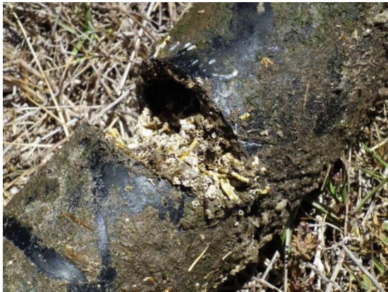
FIGURE 4.1: GROWTH OF ORGANISMS CLOSING CTD TUBES.
