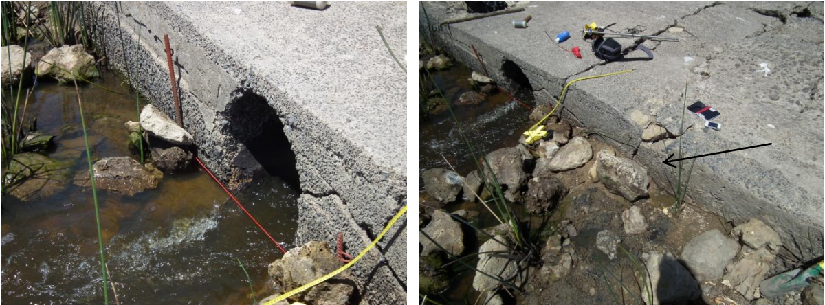
FIGURE 3.10: CONSTRICTIVE POINT USED FOR DISCHARGE MEASUREMENTS.
