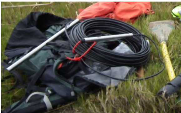
FIGURE 3.1: OTT CTD DIVER. THE PROBE IS ATTACHED TO A LONG CABLE WHICH ENDS WITH THE READER UNIT WHICH CAN BE BURIED NEXT TO THE RIVER.
