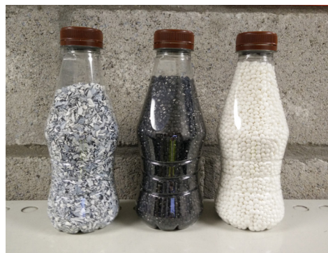
Figure 2.19: Granulate used for production HDPE bottles. Inner layer - middle layer - outer layer
