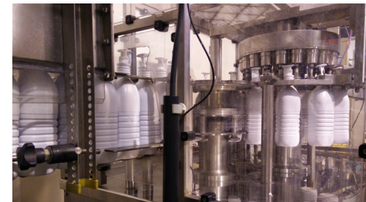
Figure 2.23: Head trimming machine where head is removed
