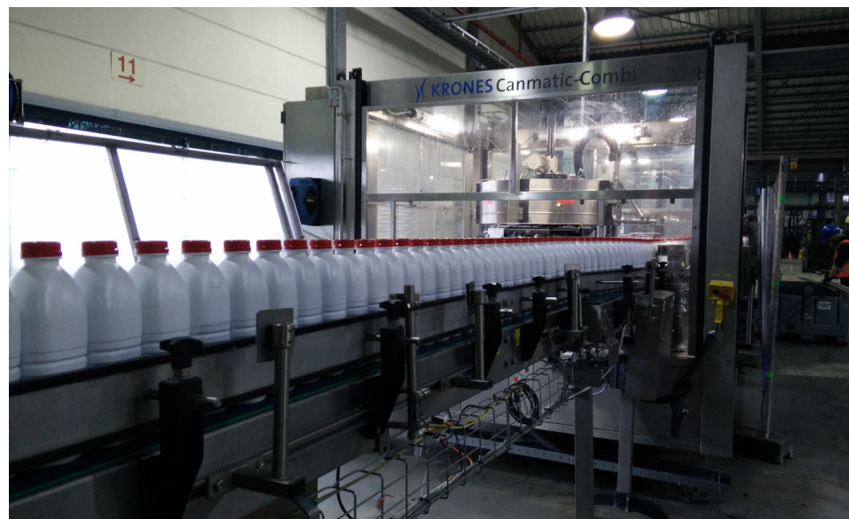
Figure 2.25: Bottles with cap just before the labelling machine
