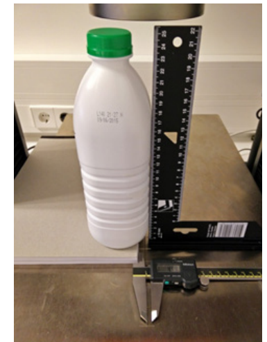
Figure 2.5: Measuring method for overhang simulation
