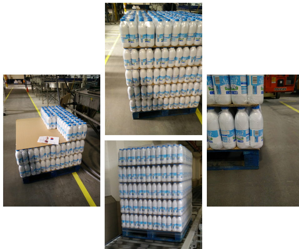
Figure 2.9: Building of the pallets for transport test
