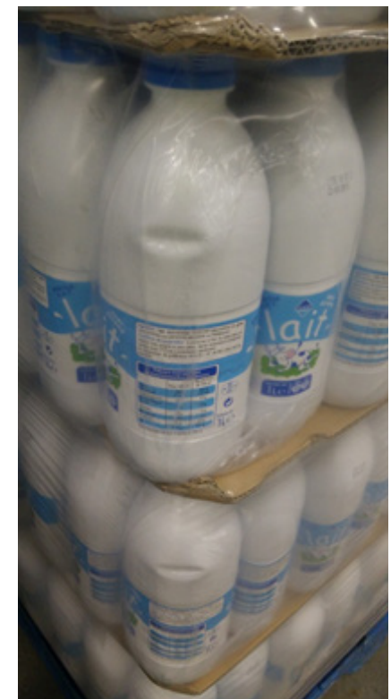
Figure 2.12: Dents on bottles in the corner of the pallet
