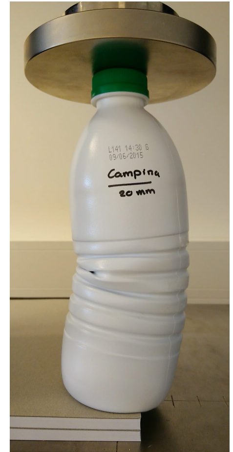
Figure 2.7: Effect of overhang by top load applied on a bottle
