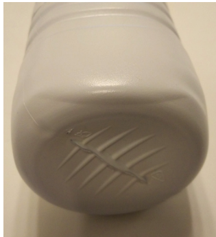
Figure 2.6: Example of damage on a bottle after test (Campina > 7,5mm overhang)
