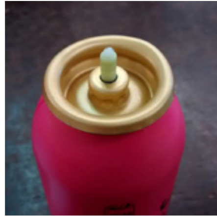
An example of an aluminium pressurized can male valve. This type of valve needs an actuator which will be around the valve.
