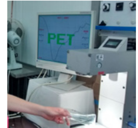
NIR-scanner to identify the material of the bottle: PET. The machine shows the graph of the absorption and reflection. The machine indicates the material.
