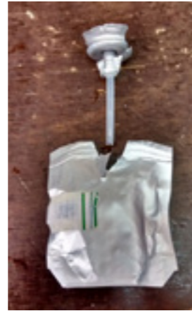
The aluminium pressurized can bag on valve. The valve, basis, pipe and bag can be seen.
