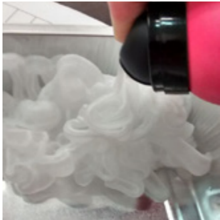
Emptying an aluminium pressurized can. The gel does not directly turn into foam because the temperature is not high enough to boil the pentane inside the gel.
