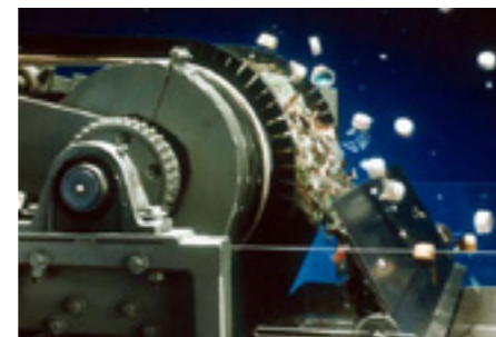
Figure 41 - Eddy current separator, remover non-ferrous materials
