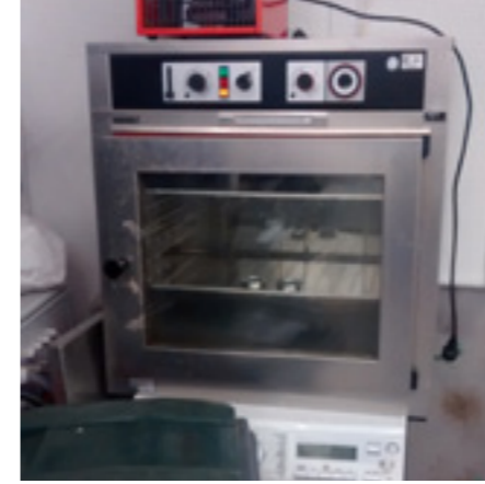
The oven used for the oven test to detect the material which cannot be detected by the NIR scanner
