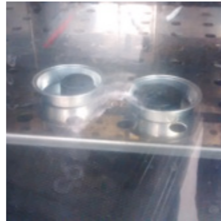
Put the two caps in the oven at a temperature of 130°C for one hour.
