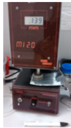
The machine, Adamel Lhomargy MI 20, to define the thickness of the bags of aluminium pressurized cans and soups pouches. In this picture a bag of aluminium pressurized cans is measured.
