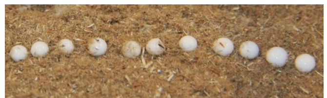
Figure 15. Droplets of binder on a sawdust powder bed
