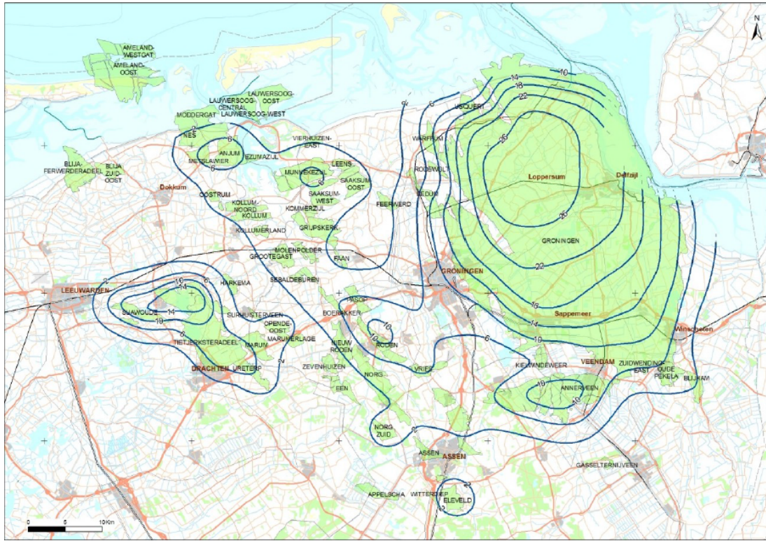
FIGURE 2.2: Illustration of the ground subsidence since the start of the gas extractions in 1964 (NAM, 2010).
