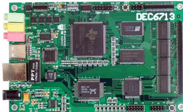
Figure 10: A digital signal processor
