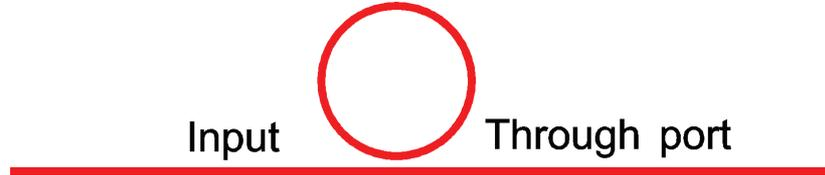
Figure 5: Schematic representation of a microring resonator (MRR). Light from the input is coupled in and out of the MRR with a directional coupler.
