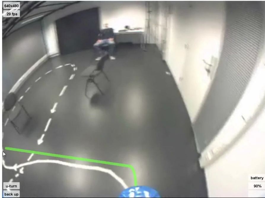
Figure 21. While the participant was turning left, he moved the mouse pointer out of the left video boundary and that made the robot stop. This behavior was only shown with the mouse
