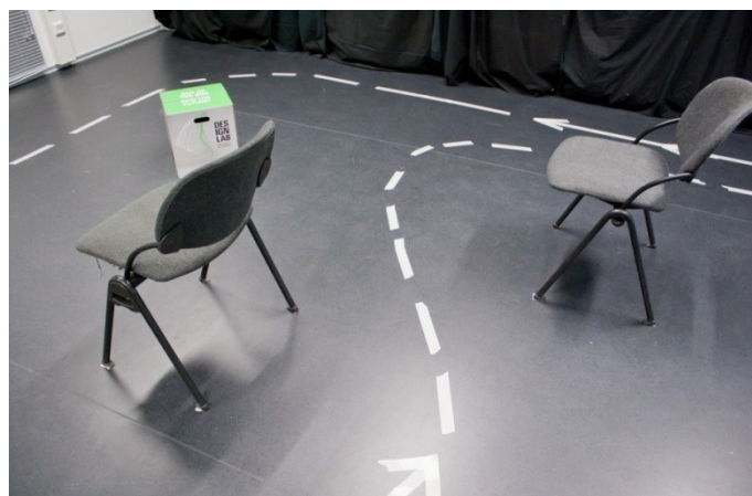
Figure 7. The distance between the last two chairs in the driving path was 84cm. That was small enough to simulate passage through a doorway
