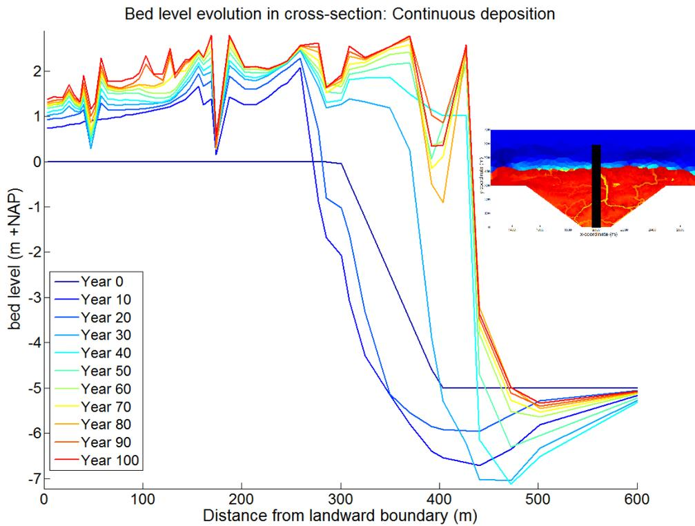
FIGURE 25 BED LEVEL DEVELOPMENT FOR SIMULATION WITH CONTINUOUS DEPOSITION. THE BLACK SOLID LINE IN THE SMALLER FIGURE REPRESENTS THE LOCATION OF THE CROSS-SECTION
