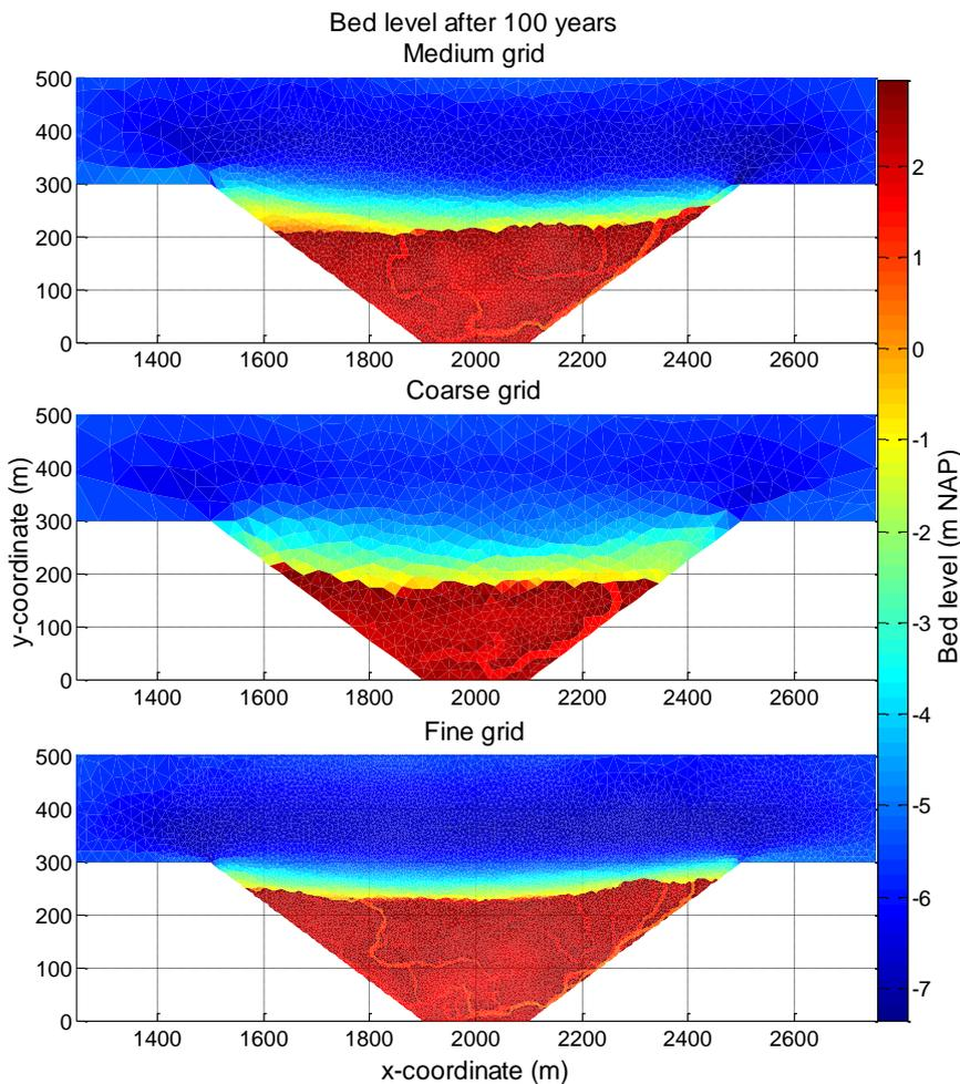
FIGURE 39 BED LEVEL MEDIUM, COARSE AND FINE GRID
