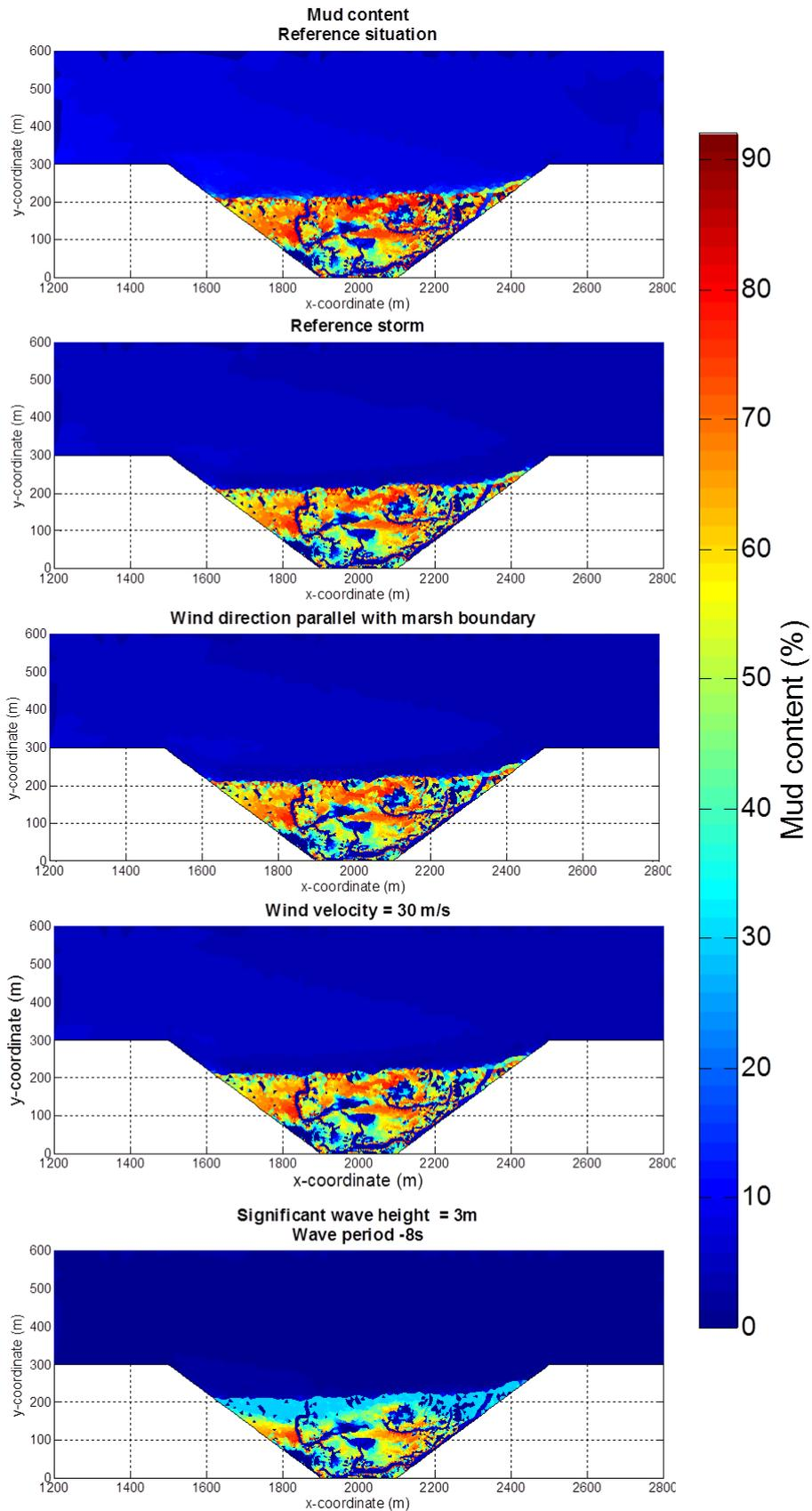
FIGURE 32 MUD CONTENT AFTER DIFFERENT STORMS. IN THE UPPER FIGURE, THE INITIAL MUD CONTENT BEFORE THE STORM IS PRESENTED
