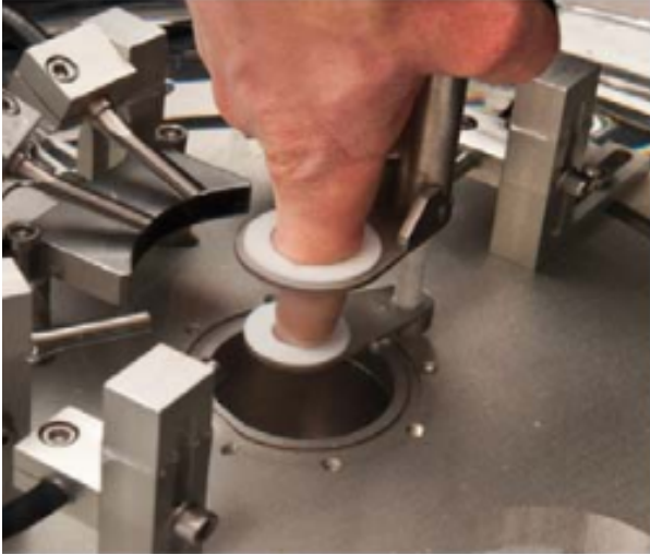
Figure 1: Photoacoustic tomography system This figure shows the photoacoustic tomography system doing a measurement on a human finger. A schematic version of this setup is later shown in Figure 3 & Figure 6 .
