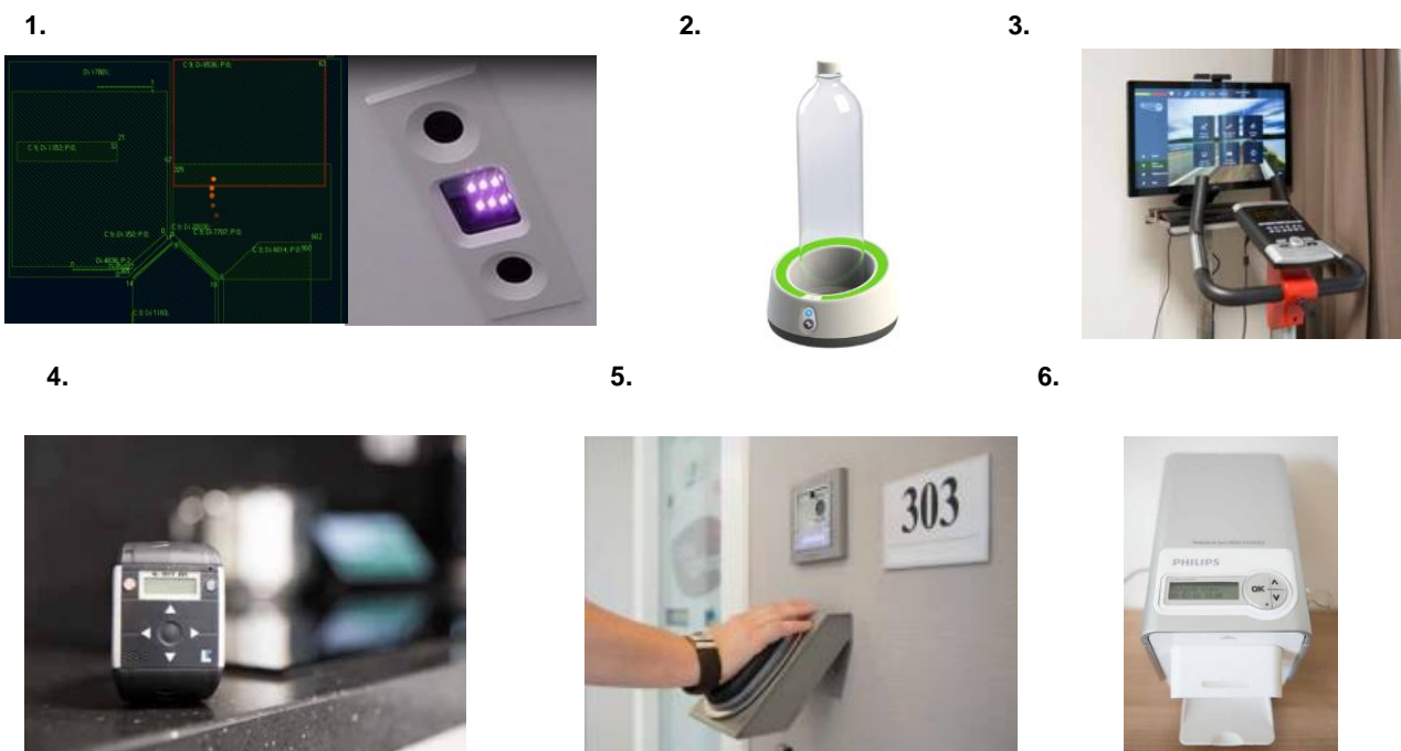
Figure 3: Smart Home sensors: infrared sensors (1), Obli; registers fluid intake (2), home trainer (3), Smart watch (4), palm scanner (5), Medido; automatic medicine dispenser (6)
