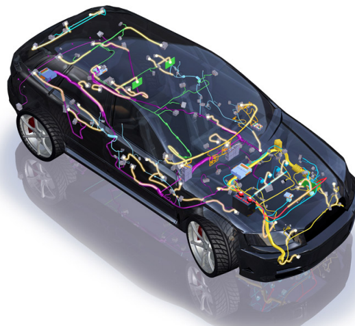
FIGURE 7: ECU's in a car. Image from (Delphi, 2012).
