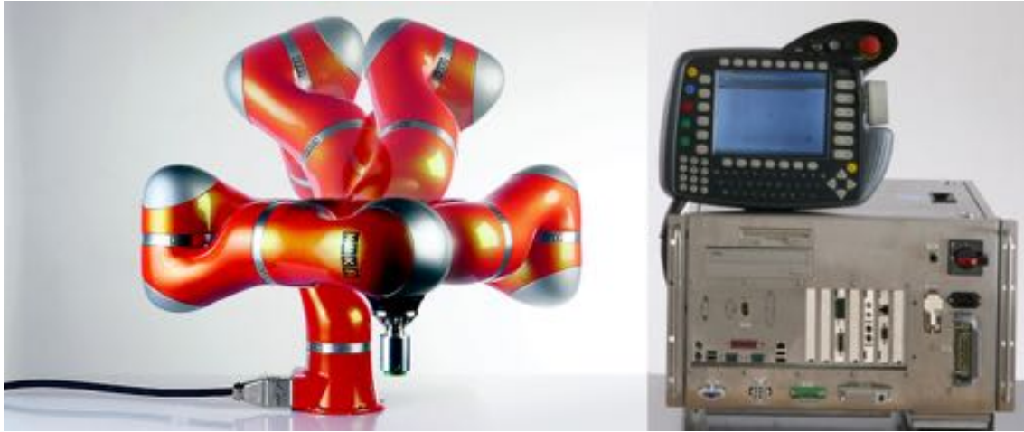
Figure 3.6: (left) KUKA LWR4+, (right) KRC controller
