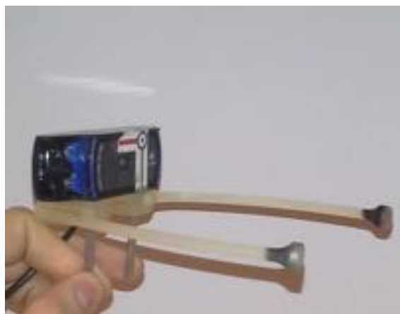
Figure 3.14: Camera mount and magnetic grabber
