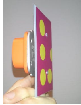
Figure 3.10: Marker plate with IMU backplate
