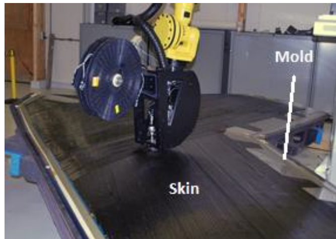
Figure 2-1. AFP placing the skin on top of the mold by robot for a prototype
