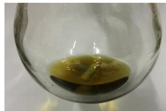
(b) Photograph of the phenolate anion of 4'-hydroxybenzo-18-crown-6 in THF, generated using a phosphazene base
