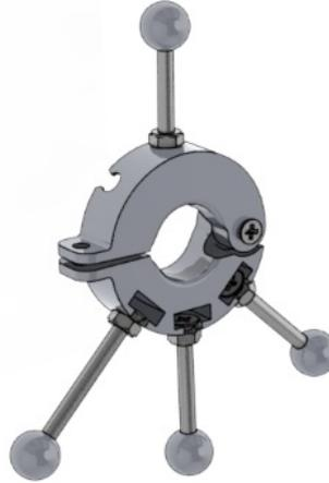
**Figure 3.1:** The holder for the OptiTrack balls which is mounted on the tip of the endoscope. The design is optimised for 3d printing, it consists of two parts which are identical and can be printed without overhang. The inner diameter is wider around the pivot and clam, preventing any damage to the endoscope during tightening. The shaft with the OptiTrack balls are modular to test different configuration such as lengths. The final shafts are made from aluminium limiting the weight.
