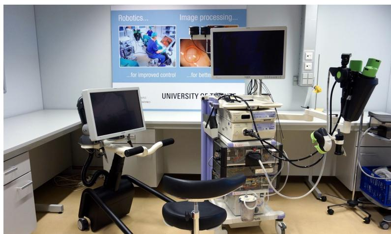
**Figure 1.1:** The TeleFLEX setup. An endoscope is mounted in the steering module which can be seen in the right..
