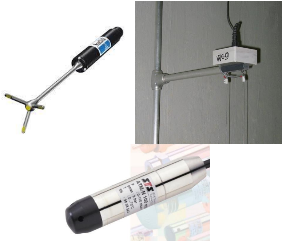
Figure 3.5: Upper left: Acoustic Doppler Velocimeter. Retrieved from: SonTek, upper right: Resistive Wave Gauge. Source: Van der A & Cáceres (2015), Bottom: Pore Pressure Sensors. Retrieved from: Van der A & Cáceres (2015)
