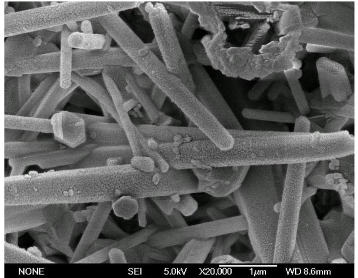
Figure 17: SEM image of a grafted  $\text{Si}_3\text{N}_4$  membrane. The change in morphology, the tiny white dots, are clearly present
