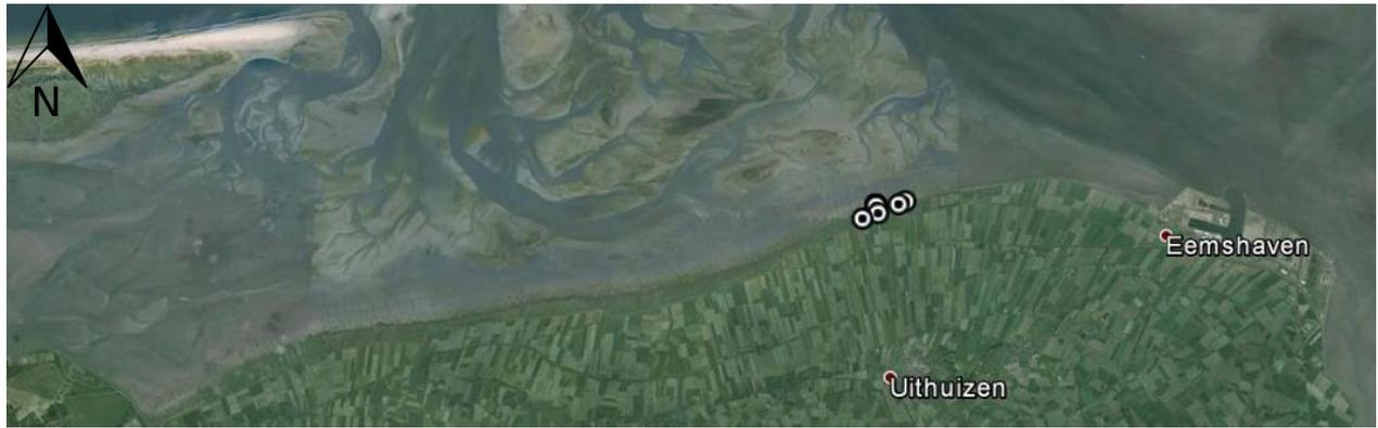
Figure 14 Area of interest near Eemshaven, The Netherlands. Salt marshes seen on the left, sandy foreshore on the right and a transition zone in the center of the figure. The locations of the pressure gauges are shown by the icons.
