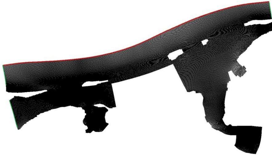
**Figure 38** Flow boundary locations. The northern (red) boundary dictate a water level, green boundaries dictate flow in and out of the boundary. The missing square is filled by the refined grid.
