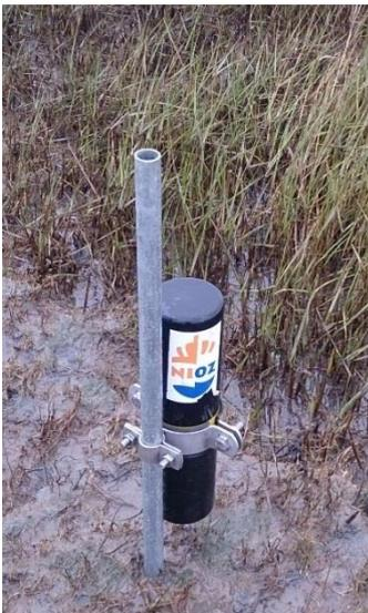
The waves and water level on the marsh were measured with pressure gauges which were dry during low tide and inundated during high tide. The pressure gauges had a certain height from the bottom which means that water depths below approximately 0.2 meters were not registered (Figure 16). These measurements can be seen in Figure 17.
