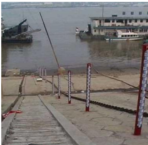
Figure 4.4 inclined staff gauge, Yangtze River
