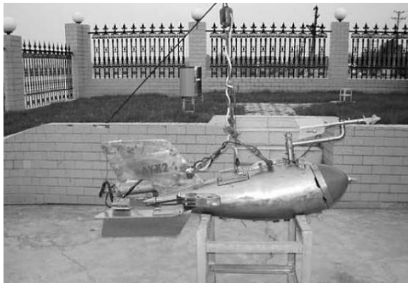
Figure 4.11 Combined sediment sampler, current meter, sinker weight and ultrasonic depth gauge
