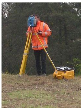
Figure 4.2 Total Digital Station in use
