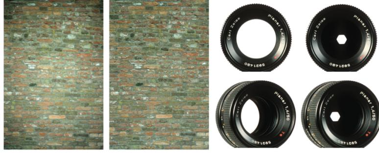
Figure 2.2 - [10] Two images of a wall, taken with different diaphragms. The aperture of the lens changes with the angle of incidence.
