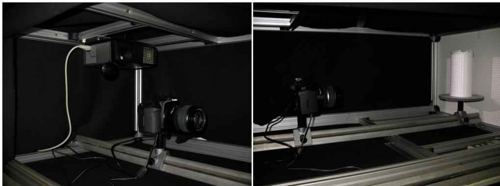
**Figure 3.1 – Photographs of the structured light rig. In the left image the projector and camera can be seen. In the right image a platform can be seen that holds an object to reconstruct, in this case a cylinder. As an example, a grid of lines is projected onto the object.**
