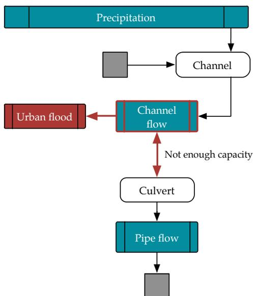
Figure B.3: Drainage system failure due to low capacity of the culvert
