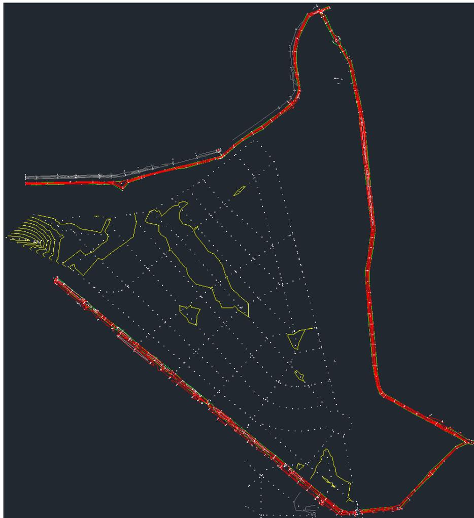
Figure 3.4: A map of the Delta del Tigre with yellow height lines. The dots are measurement points on the roads and the red line surrounding the district represents the dyke. Based on material provided by DINAGUA.
