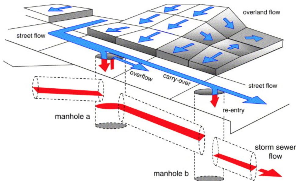
Figure 2.2: Idealised surface (blue) and storm sewer (red) flow components in dual drainage systems (M. Smith, 1993).
