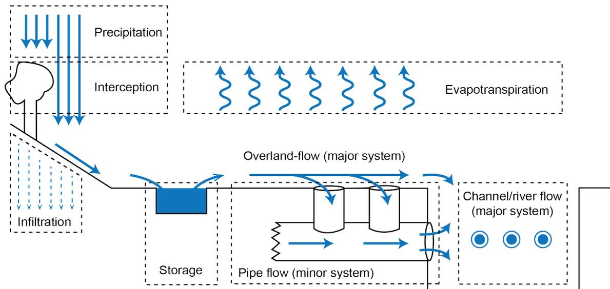
Figure 2.1: An overview of hydrologic processes during urban flooding. Groundwater flow has not been shown in the figure.
