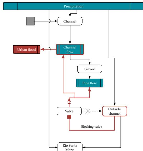
Figure B.4: Drainage system failure due to the non-return valves not functioning
