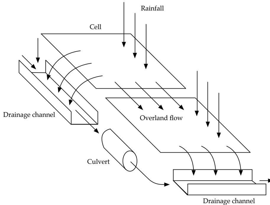
Figure 4.3: Overview of the interaction between plain cells and the drainage layer.
