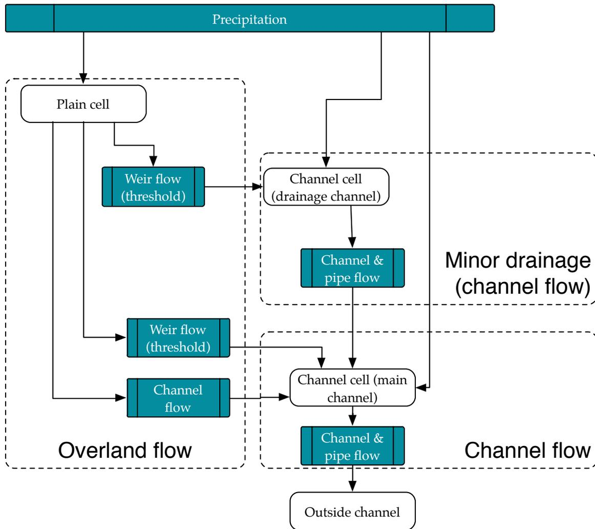
Figure 4.5: Visualisation of model structure, where green cells are the hydrologic processes and white cells the elements in the study area.
