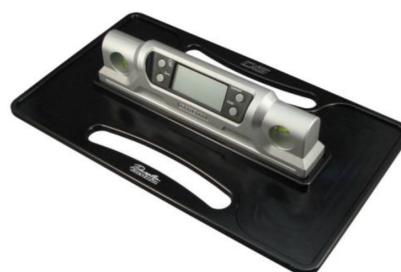
Figure 4: Official measuring device to check saddle inclination
