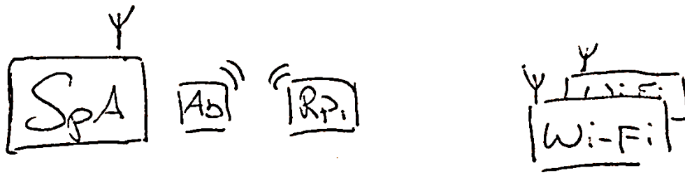
Figure 5: Sketch of the measurement setup consisting of a spectrum analyser (SpA), the wireless sensor Abel (Ab), the Raspberry Pi with Bluetooth adapter (Rpi) and the Wi-Fi routers (Wi-Fi).
