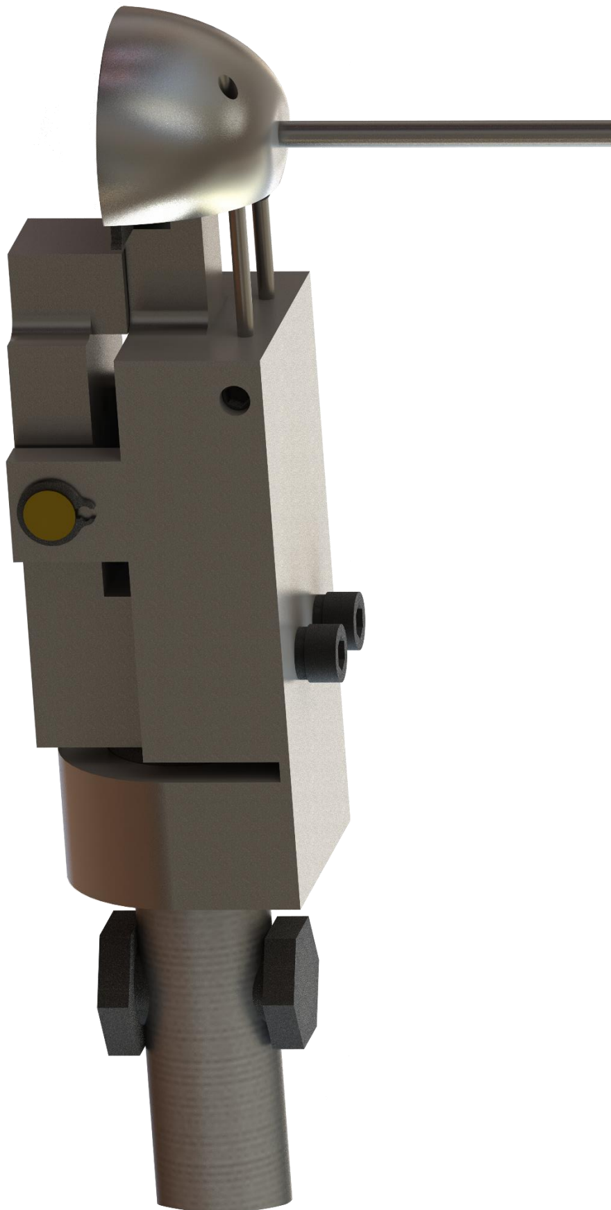
Figure 19: 3D render of the final design of the sample introduction system and the sample holding system.
