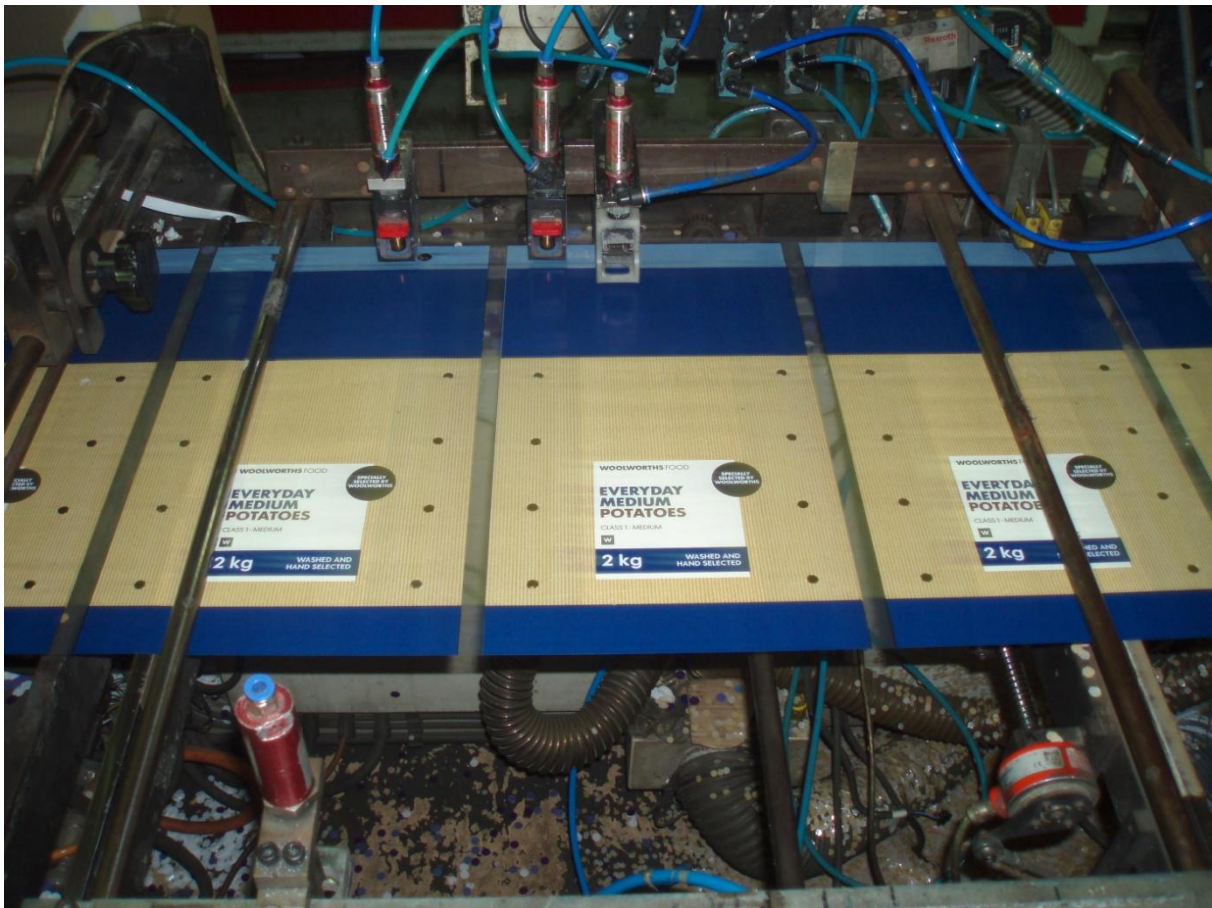
Figure 6 – Punching of wicket holes
