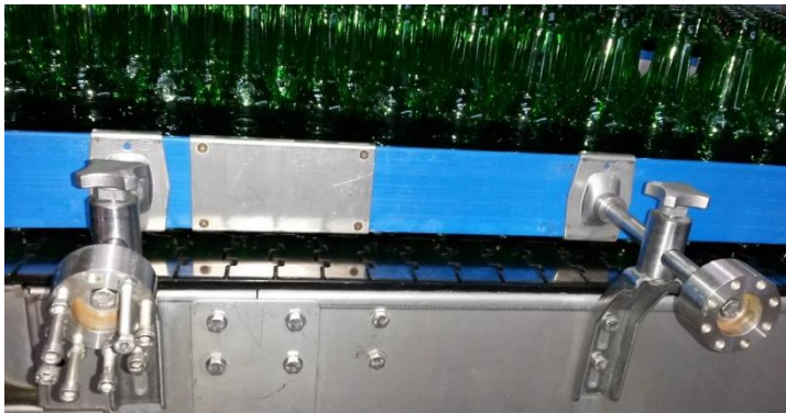
Figure 25: Left: old adjustment tools for the side barrier.
