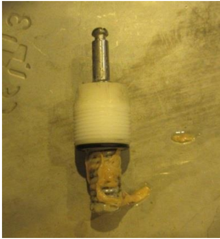
Figure 13: Dirty inside of a nozzle
