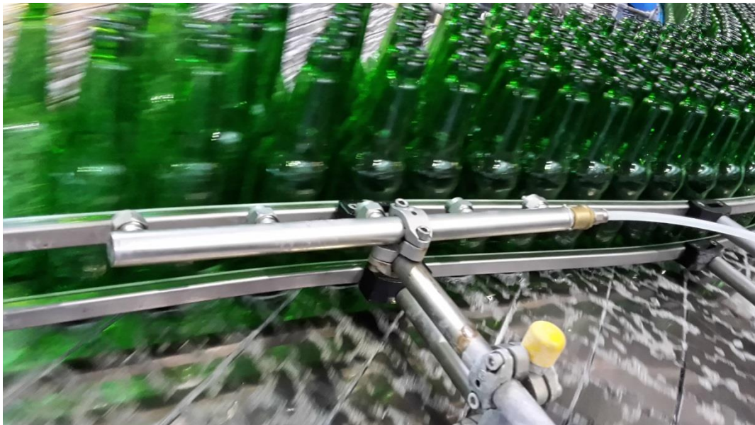
Figure 26: New spray nozzles
