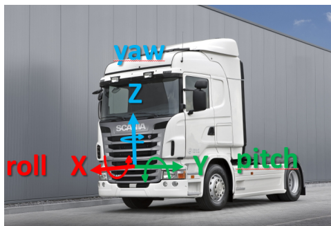
Figure 2.1: ISO direction definition[3]
