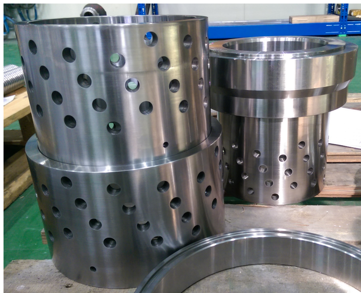
Figure 5.2: Picture of the finished cages after production. Leftbottom - Outercage (3) above it - Middle cage (2) and right the inner cage (1)
