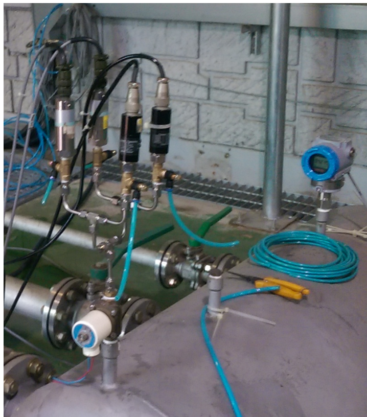
Figure 4.14: Overview of the setup used for the pressure gage calibration
