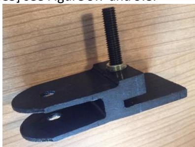
**Figure 9.7** The 3D printed component of which the screw clamps the mirror on to the edge.
