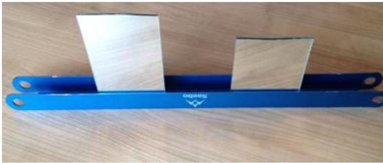
**Figure 9.5** The metal slit with the two mirrors, the left one for the camera and the right one for the projector
