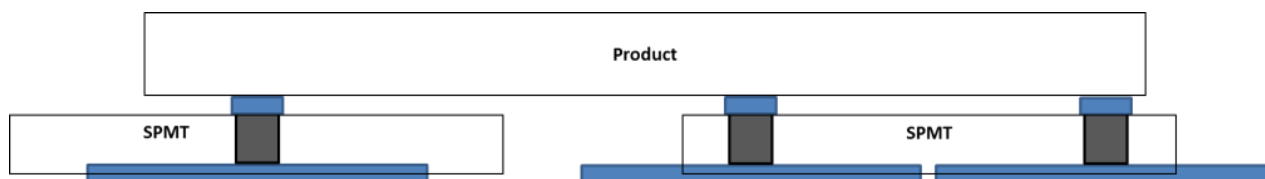
Figure 4: Three complete SSs are transported by use of two single SPMTs
