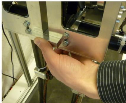
**Figure A.2:** Use the T-shaped tool to perform the hip homing.
