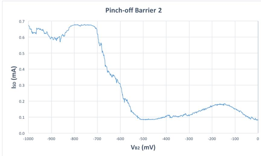
**Figure 4.14:** Pinch-off characteristic curve of  $B_2$  measured at  $T \approx 4.2$  K for a bias voltage of  $V_{SD} = 1$  mV.
