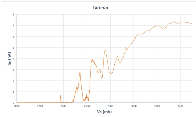
**Figure 4.1:** Turn-on characteristic curve measured at  $T \approx 4.2$  K and for a bias voltage  $V_{SD} = 1$  mV. A gate voltage  $V_G$  is applied simultaneously to all gates on the electron operation region, while the hole operation region is kept at zero voltage.
