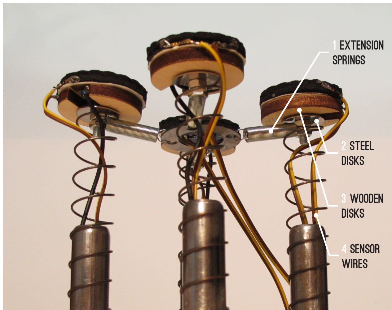
Figure 4.14 Fully assembled mechanical prototype
