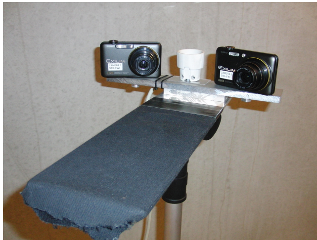
Figure 8.1: The old setup consisting of two consumer model cameras mounted on a tripod. There is a fitting for a light source.
