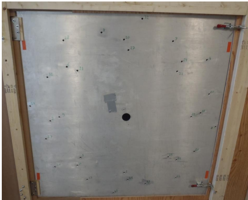
Figure 4.3: Close-up of the microphone array plate. The plate acts as a door and can open to the inside. The door is closed tightly by the clamps seen on the right of the picture. The groove in which the door fits is lined with sealant to create a sealed sound environment. The array holes are lined with simple cell phone speakers.
