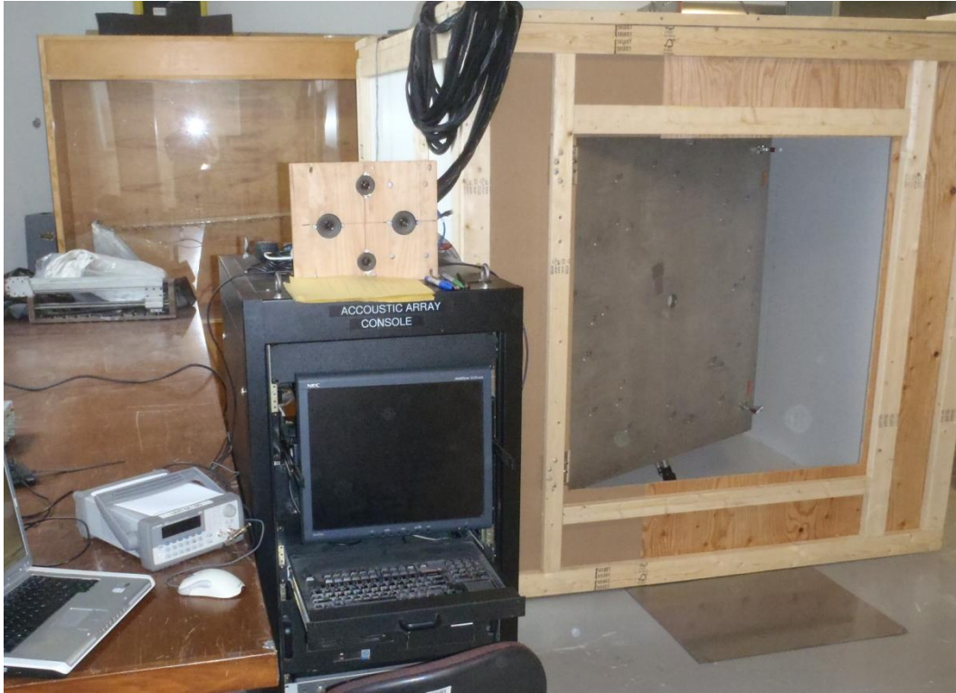
Figure 4.7: Overview of the test setup with the waveform generator on the left, the acoustic array console in the middle and the acoustic box on the right
