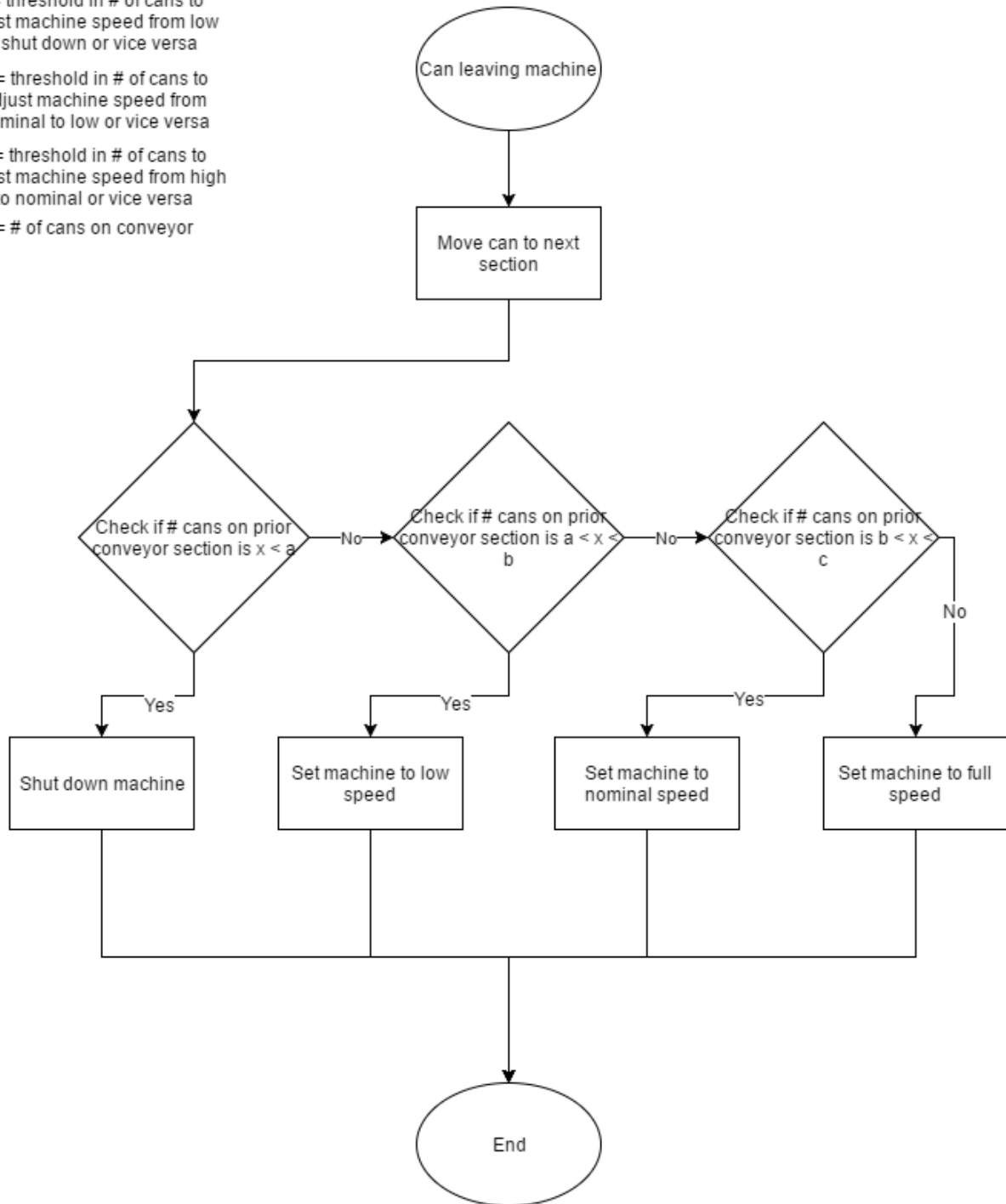
Figure 34: Flowchart of the method to determine machine processing time
