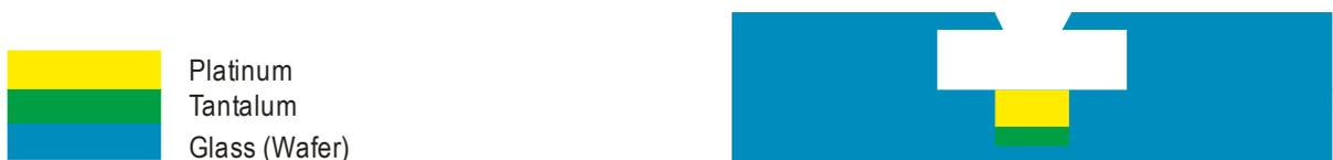
Figure 53 Wafer bonding. The two wafers on top of each other. This is the final structure.
