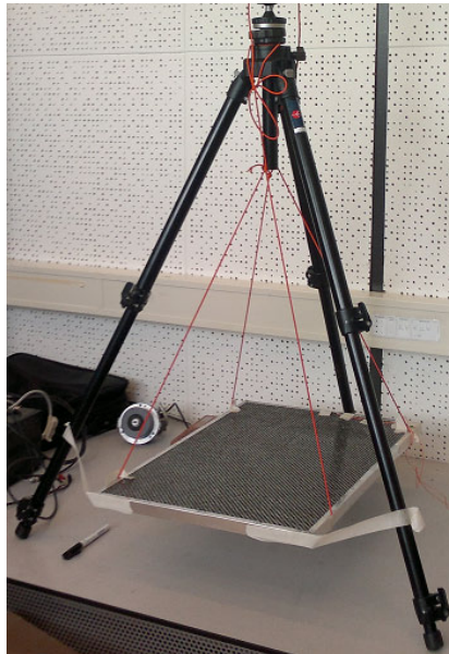
Figure 5.2: Setup for uncoupled structural measurements
